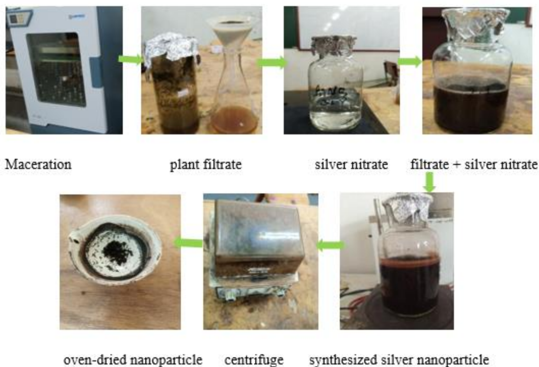
Figure 4. Silver nanoparticle synthesizing process
