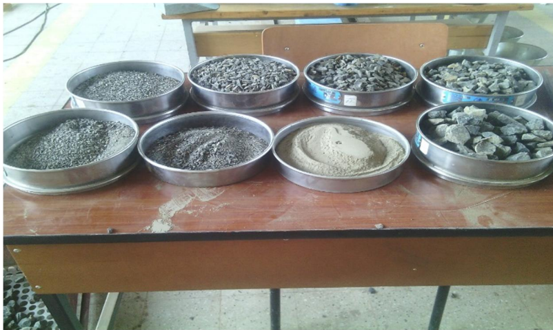
Figure 4.1 Gradation of weak Aggregate
