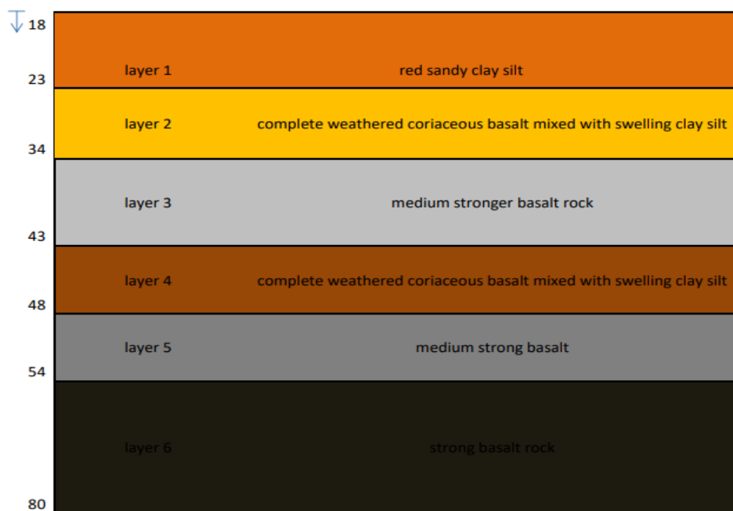
Figure 11: soil profile below the foundation level
