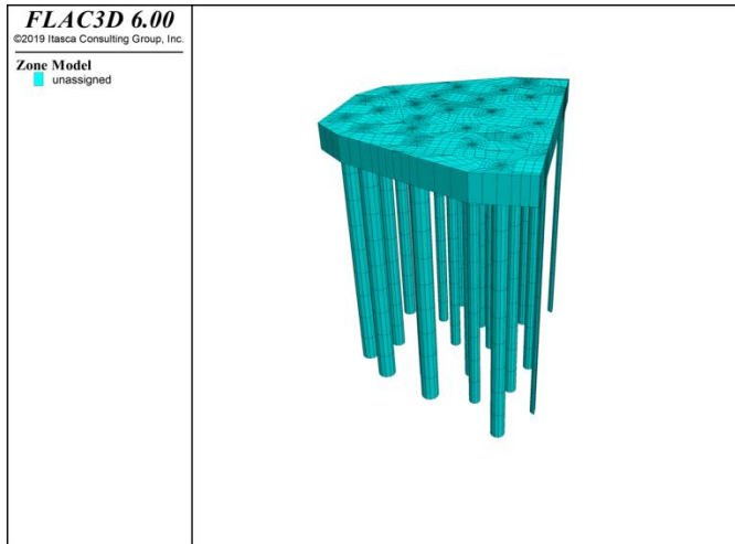
Figure 17: Pile installation step (enlarged view at pile and raft location)
