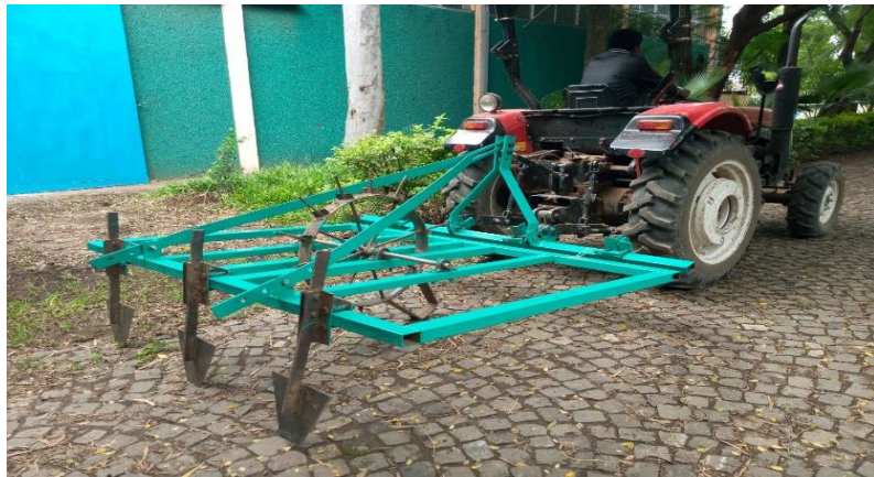
Figure 3.14. Fabricated tractor drawn tie ridger
