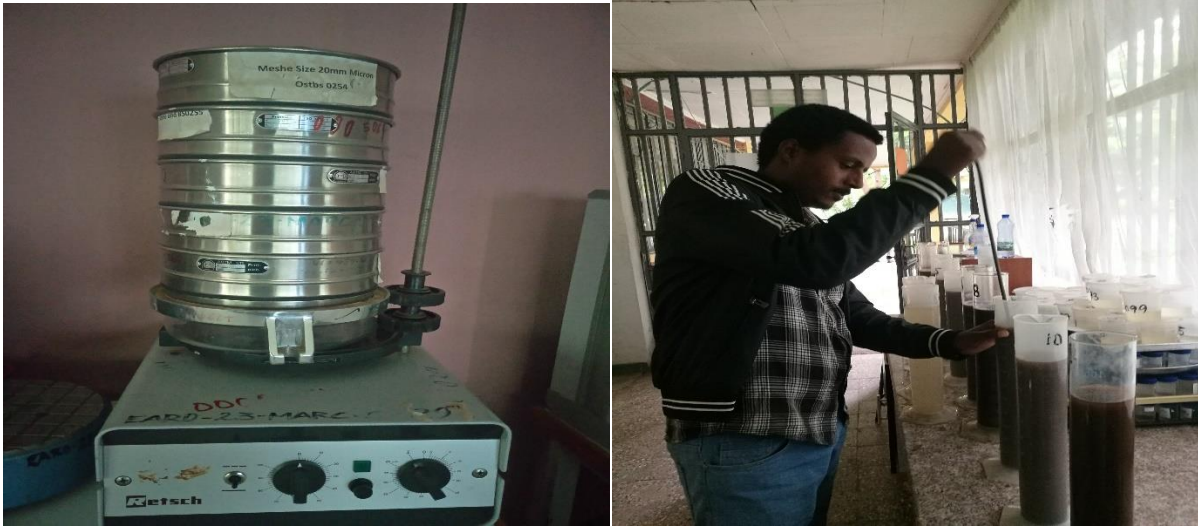
Figure 4.1. Identify the soil texture of the soil sample
