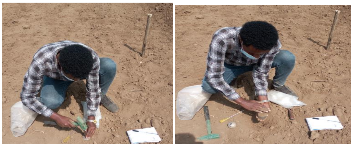
Figure 4. 3. Measurement of soil bulk density by core sampler
