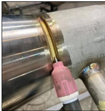
Figure 2.7. Orbital pipe welding groove (Center of Excellence for Engineers image)
