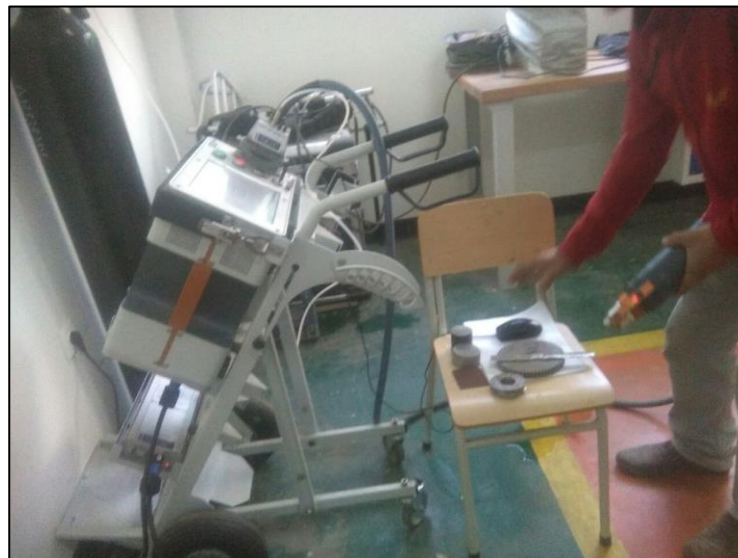
Figure 4.2. Composition analysis of SS 316 through spectroscopy
