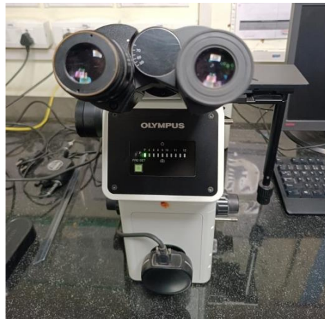
FIGURE 3. 9: OLYMPUS GX71 MODEL OPTICAL MICROSCOPE
