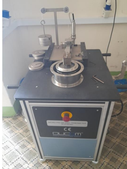
FIGURE 3. 17: MICRO PIN ON DISC TRIBOMETER (TR-20MICRO) MACHINE
