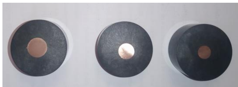
FIGURE 3. 8: C18150 MICROSTRUCTURE AND HARDNESS SPECIMENS
