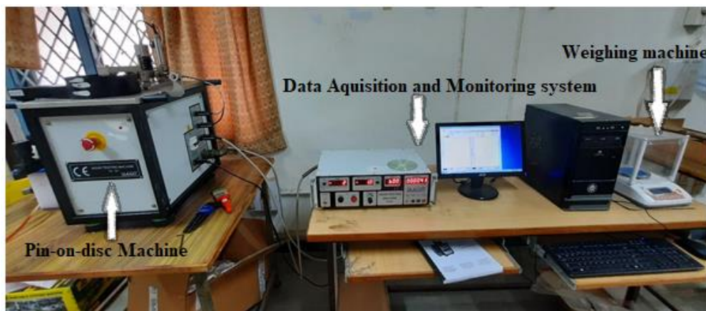
FIGURE 3. 19: PIN-ON DISK TESTING SETUP FOR C18150 ALLOY
