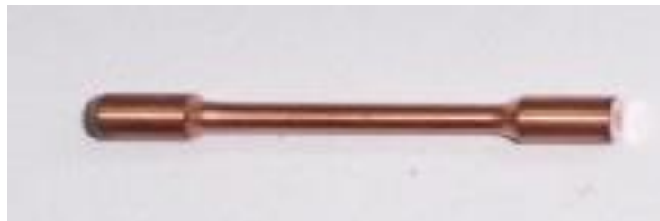
FIGURE 3. 14: TENSILE TEST SAMPLE OF A C101 ROD
