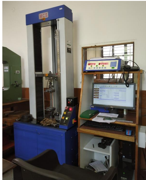
FIGURE 3. 15: MCS/UTE 20T TENSILE TESTING MACHINE
