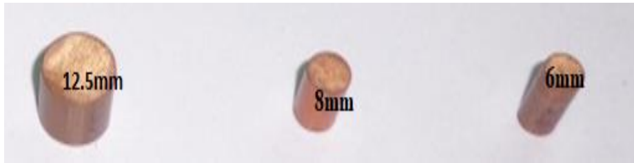
FIGURE 3. 7: MICROSTRUCTURAL AND HARDNESS TEST SAMPLES OF C101
