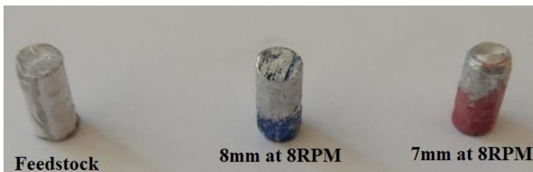
FIGURE 3. 18: AA1100 SAMPLES FOR WEAR TEST
