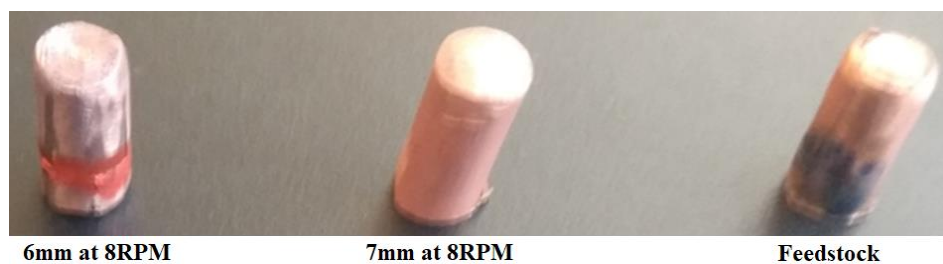
FIGURE 3. 19: C101 EXTRUDATE SAMPLES FOR WEAR TEST
