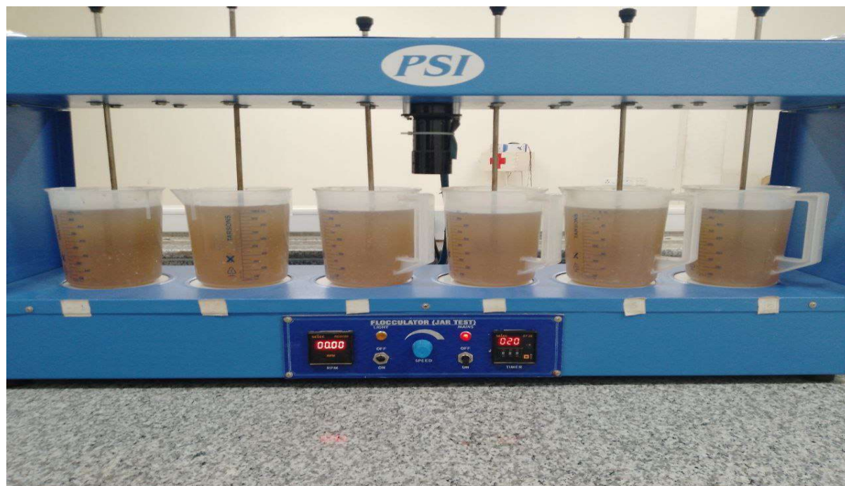
Figure 4. A photo illustration of the Jar test apparatus's experimental setup
