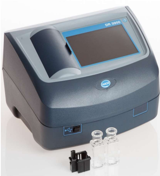
C) HACH spectrophotometer (model DR 3900)
