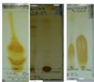
Figure 24. TLC profiles of n -hexane, chloroform, chloroform: methanol (1:1), methanol and ethanol extracts of G. purpurascens leaves
