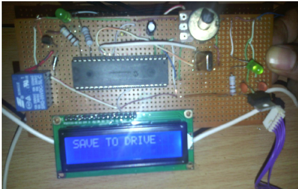
Figure 4:10 Condition when Alcohol does not detected by sensor
