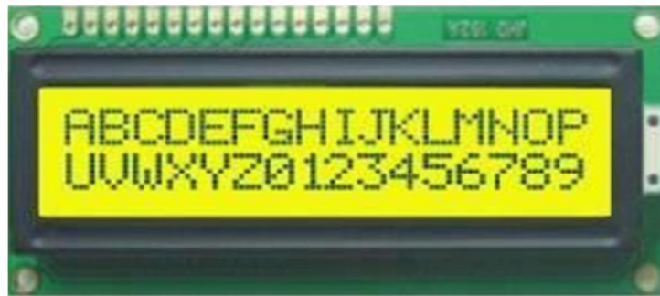
Figure 2:14 Photo of the JHD162A LCD Pannel
