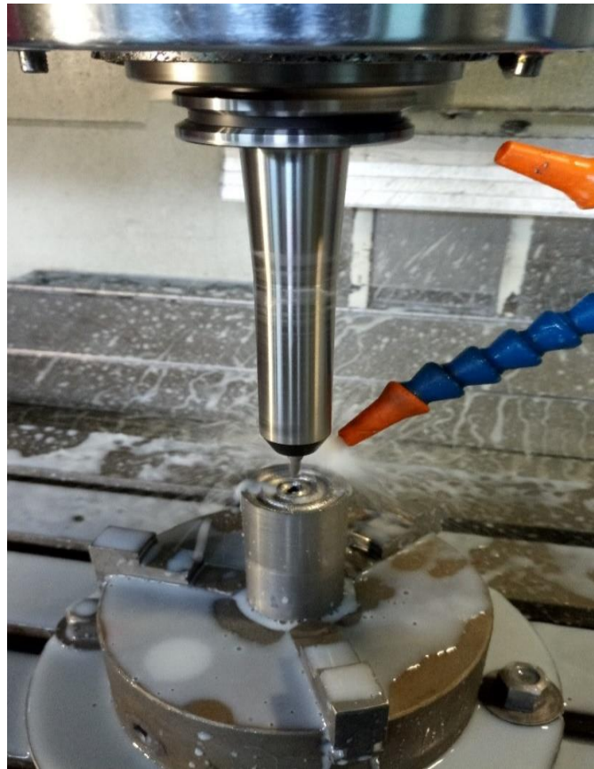
Figure 3.4 producing spiral shaped die using CNC machine
