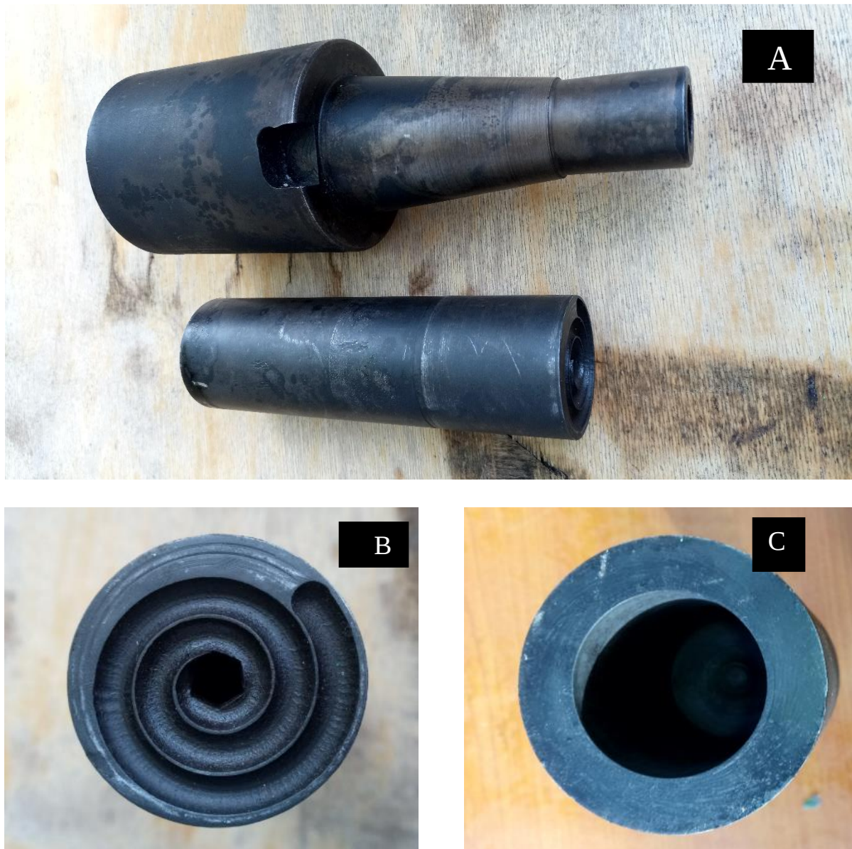
Figure 4.1 Surface of die and chamber (A), Spiral face of die (B) and Cavities of chamber(C)
