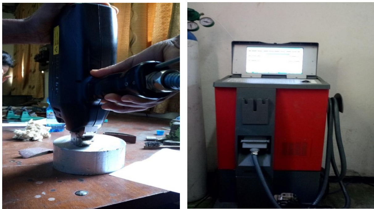
Figure 3.10 Chemical composition test instrument (spectrometer at HMMBI)
