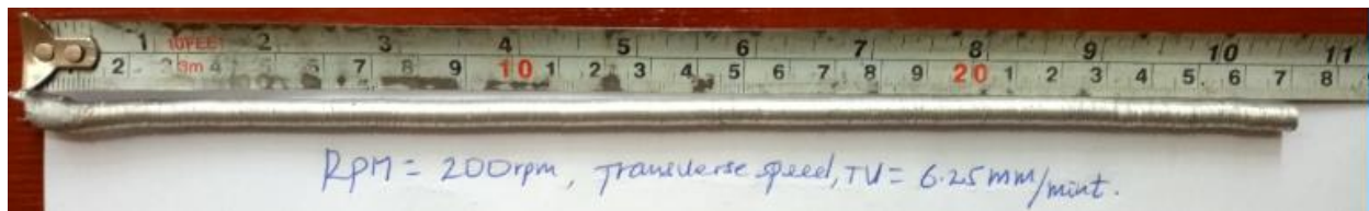
Figure 4.2 Samples extruded by friction stir back extrusion at different rotational speed.
