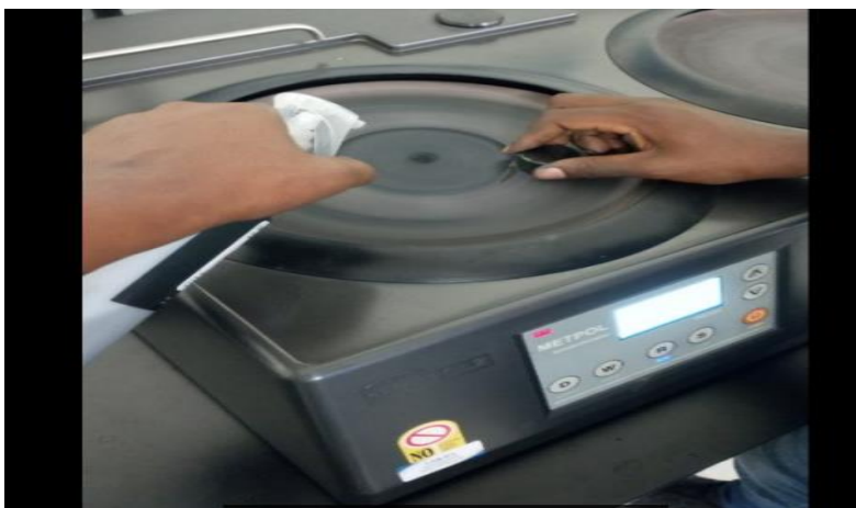
Figure 3.16 Polishing step of specimen.
