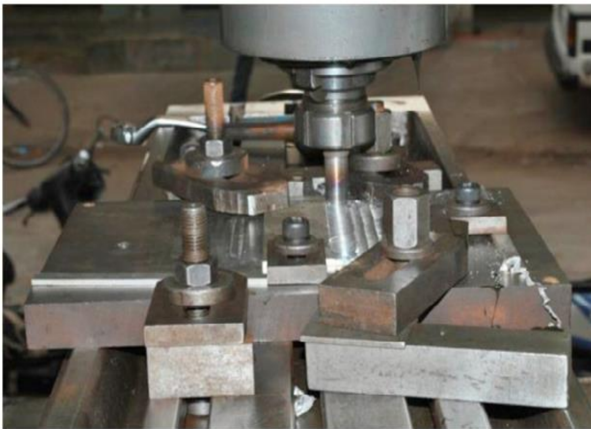
Figure.2. 9 Experimental setup of friction stir welding of magnesium plate (Babu et al. (2018))
