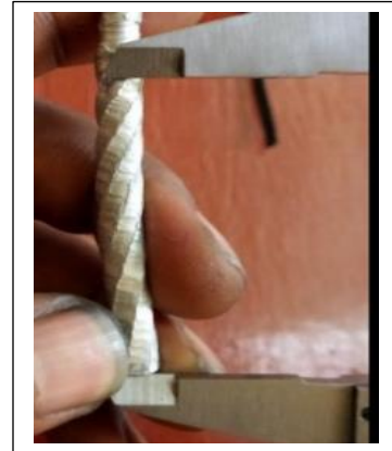
Figure 4.4 Calculation of twist angle measurement a) pythagorous b) measurement
