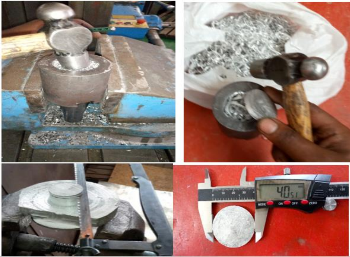
Figure 3.12 Pre compaction and Disc preparation of aluminum alloy 6063
