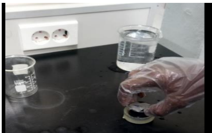
Figure 3.17 Etching of sample by HF, HNO 3 , HCl, and Methanol.
