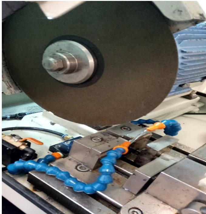
Figure 3.14 Cutting sample specimen for microstructure test by using abrasive cutter.
