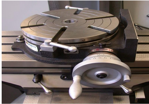
Figure 3.6 Rotary table that fixed with milling machine table (manual of Excel machine tool)
