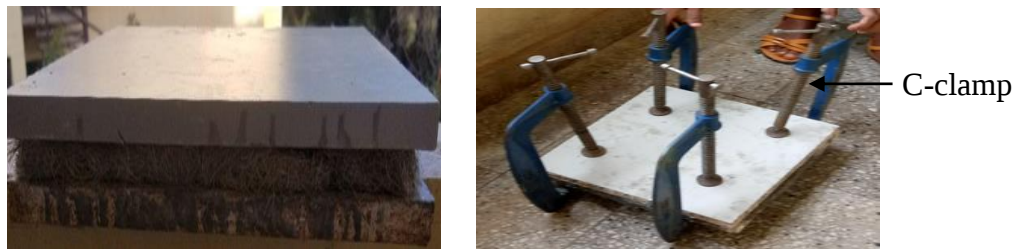
Figure 3.11 Fabrication through hand layup method
