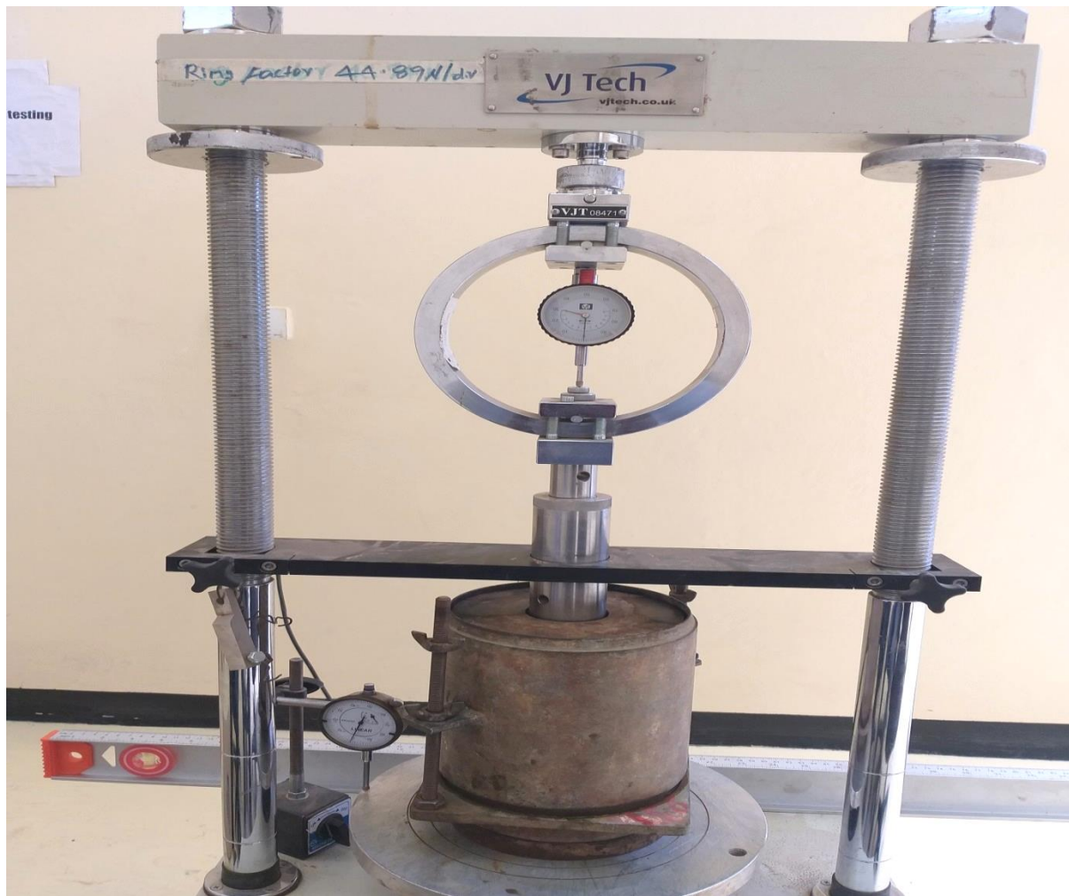
Figure 3.6 CBR stress- strain test
