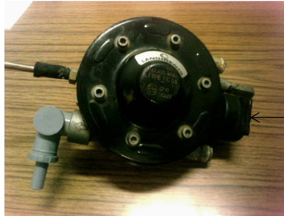
Figure 18: Electronic cut – off valve on LPG regulator
