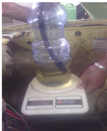
Figure 10: Measuring fuel consumption of Gasoline- ethanol blend
