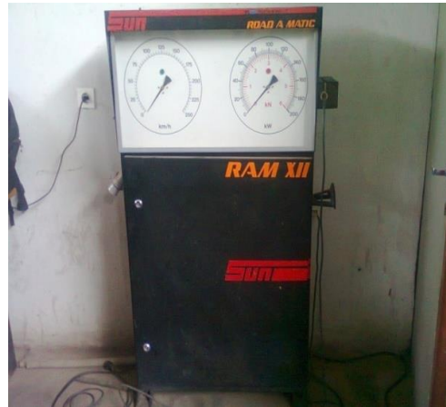
Figure 9. The sun road- a-matic XII chassis dynamometer
