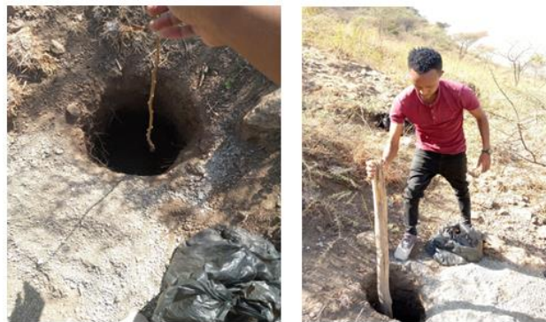
Fig 3.3: a collection of an undisturbed soil sample from depth.
