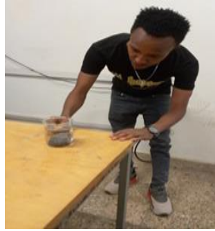
Fig 3. 2 Measuring the saturated volume of a rock sample in a Beaker filled with water.
