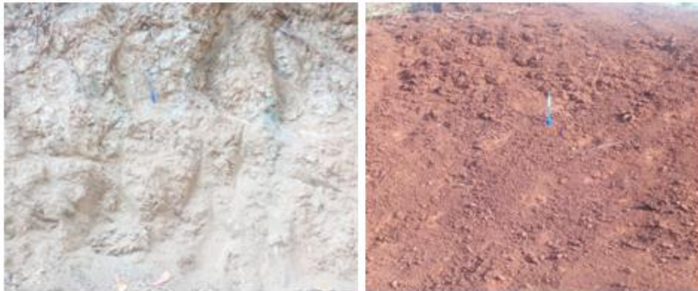
Figure 8: Exposure of alluvial soil (left) and residual soil (right)
