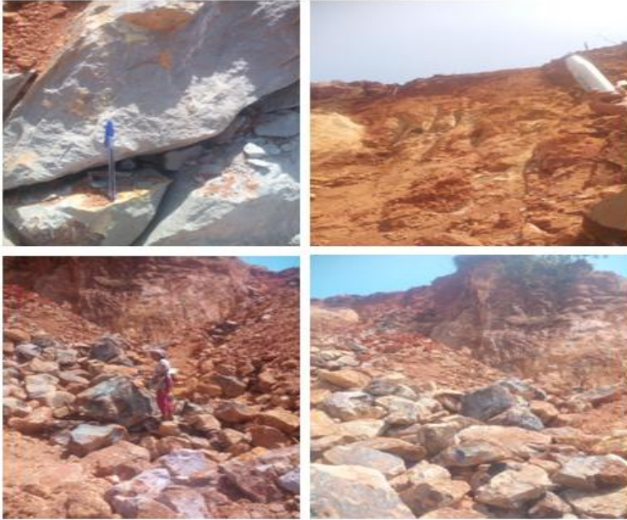
Figure 10: Fresh and weathered Ignimbrite Exposure in the quarry sites
