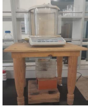
Figure 3.9 Experimental density measurements in distilled water.
