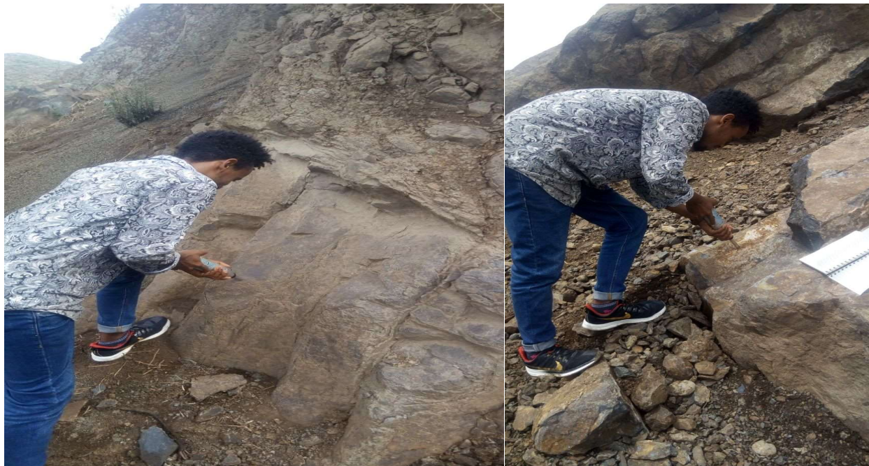
Figure 4. 1 Schmidt hammer rebound rock strength test on field.
