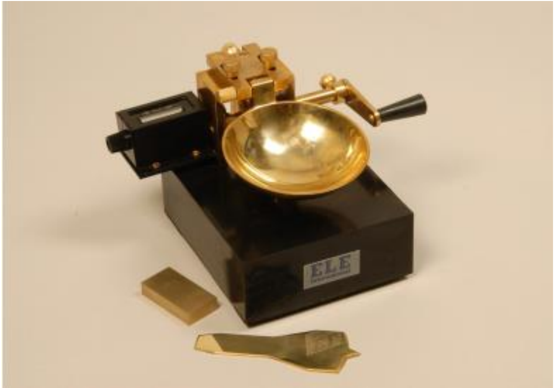
Figure 5: Percussion Method Apparatus for LL Determination (Casagrande, 1932)
