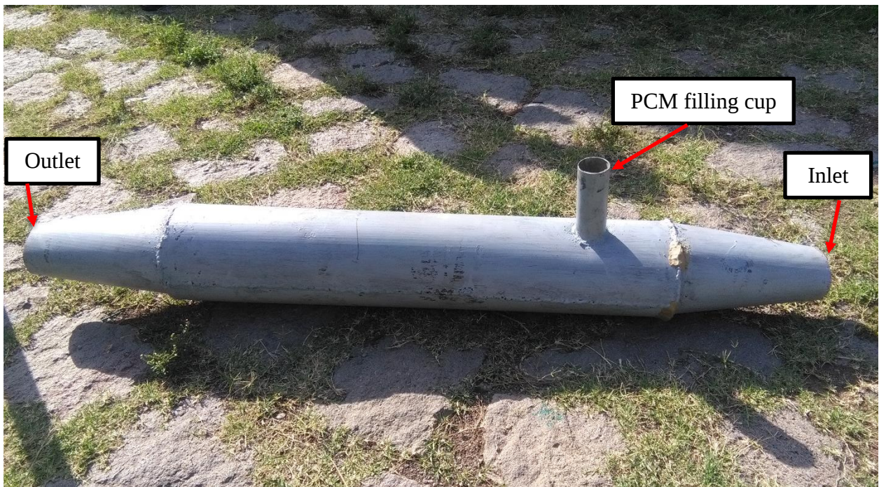
Figure 5.2: Manufacturing process of the LHS.
