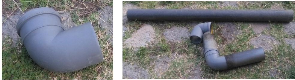
Figure 5.6: Pipe and fittings used for assembling the dryer.
