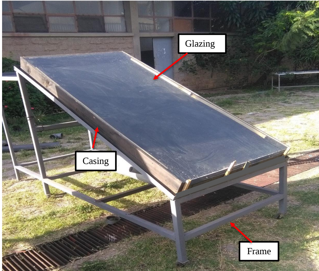
Figure 5.1: Manufacturing process (a) and pictorial view (b) of the solar air heater.
