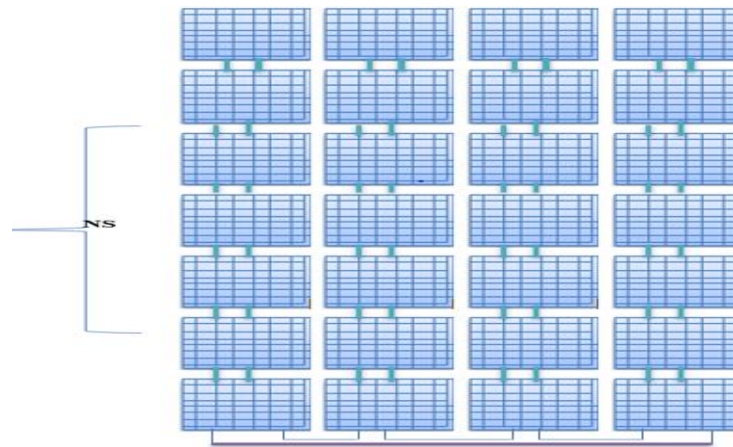
Figure 3.3 Numbers of Seven Series Modules and Four Parallel String of PV Array(Deshpande & Bodkhe, 2017)
