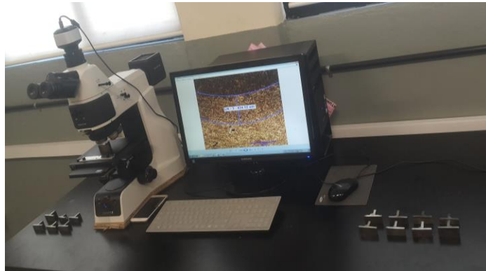
Figure 3.21: Extent of HAZ measurement (ASTU, Ethiopia)
