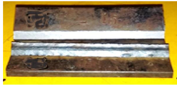
d) weldment failure pattern at 55°
