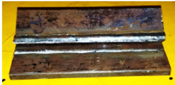
a) Weldment failure pattern at 35°
