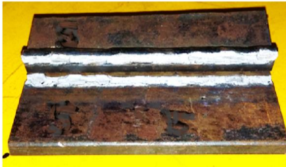
(a) Weldment failure pattern at TJ15
