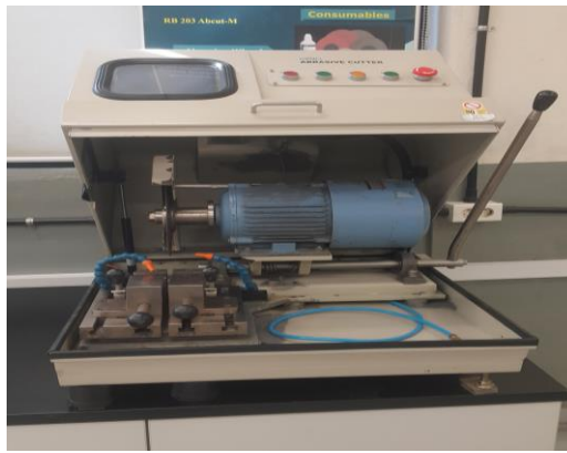
Figure 3.15: Abrasive cutting machine (ASTU, Ethiopia)
