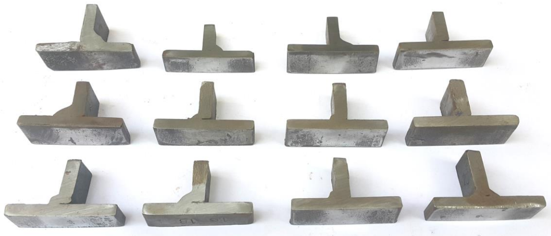
Figure 3.17: Welded specimens for mechanical test and microstructural examination
