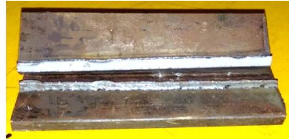
b) Weldment failure pattern at 45°
