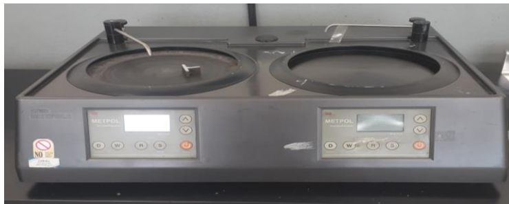
Figure 3.16: Polishing machine (ASTU, Ethiopia)
