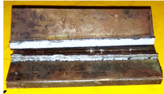
(b) Weldment failure pattern at TJ4
