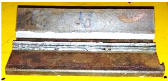
c) Weldment failure pattern at 50°
