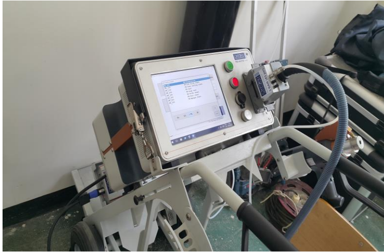
Figure 3.1: Spectrometer setup for material composition test
