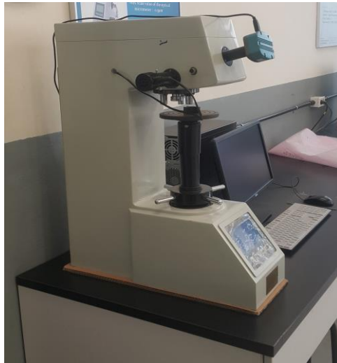
Figure 3.23: Vickers micro-hardness tester (ASTU, Ethiopia)
