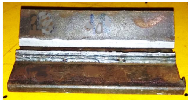
(c) Weldment failure pattern at TJ12
