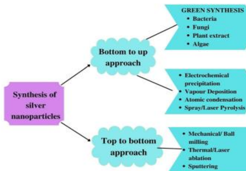
Figure 1: Synthesis of silver nanoparticles
