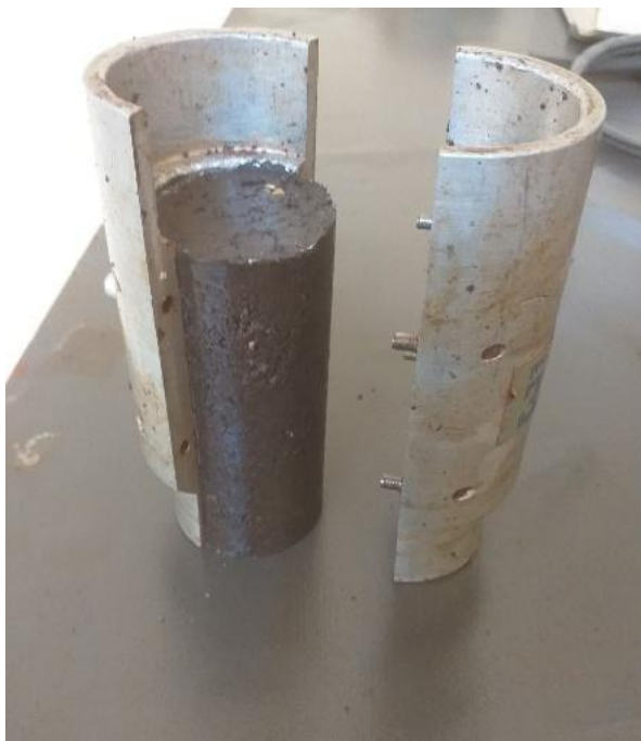
a) Sample removal for UCS test
