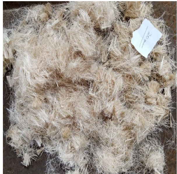
d) 20mm kerosene coated enset fiber
