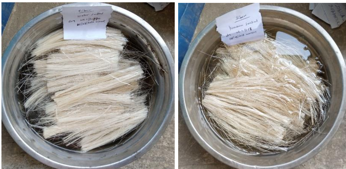
Figure 3.7 Water absorption test on uncoated and kerosene coated enset fiber
