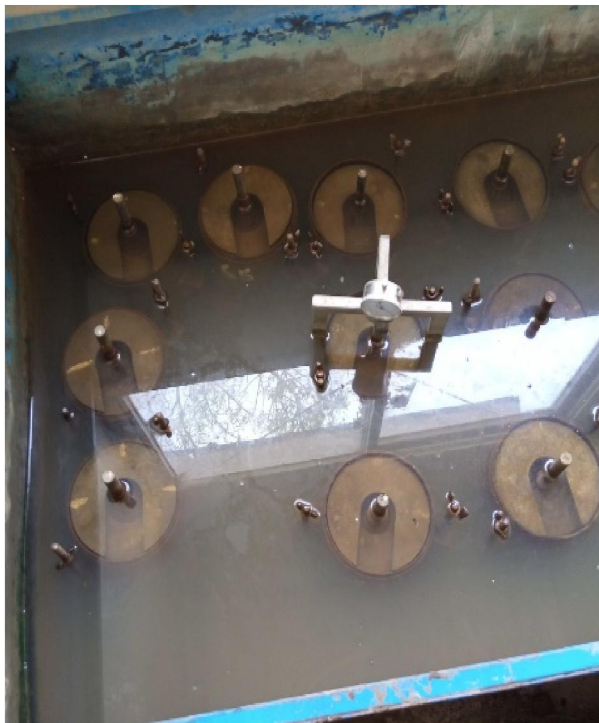
a) Soaked CBR sample with tripod in water tank
