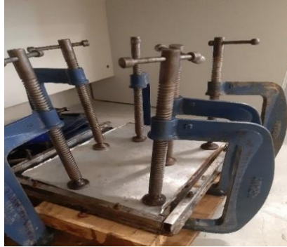
Figure 3.18 Compress and hold by using C-clamp
