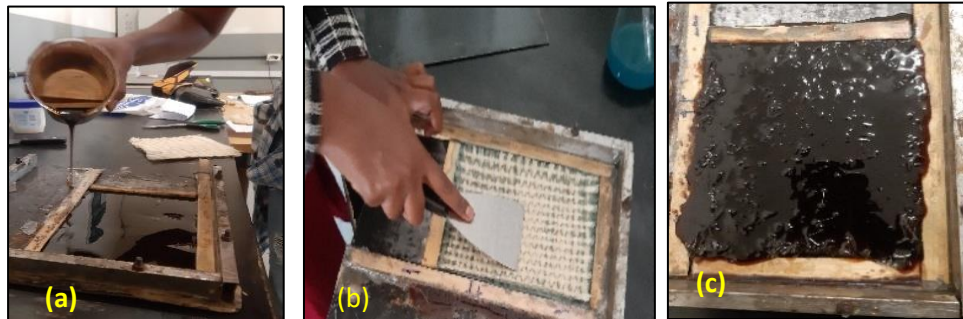
Figure 3.17 a) Add mixture on the mold b) Add PALF over the mixture c) pour the mixture over the fiber.
