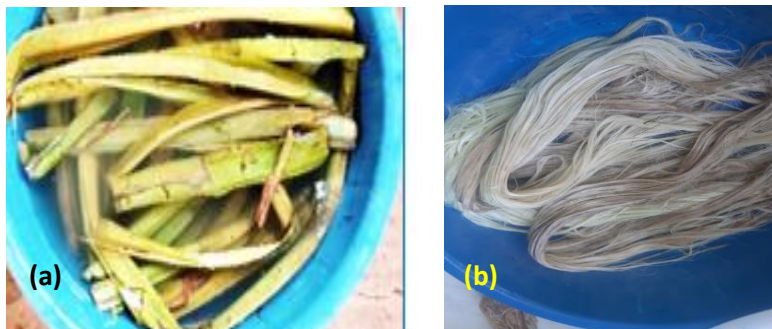
Figure 3.7 (a) Pineapple leaf and (b) Extracted pineapple leaf fiber
