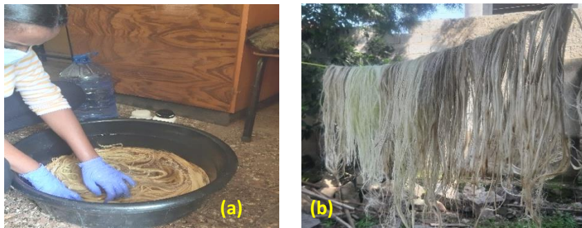
Figure 3.8 ( a) NaOH soaking of pineapple fiber and ( b) NaOH treated pineapple fiber and dried
