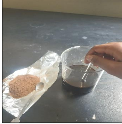
Figure 3.16 Mixture of polyester, CH, and hardener
