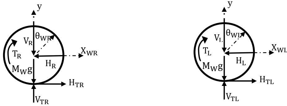
Figure 3.4:- Force Analysis of Right and left-Wheel [14].
