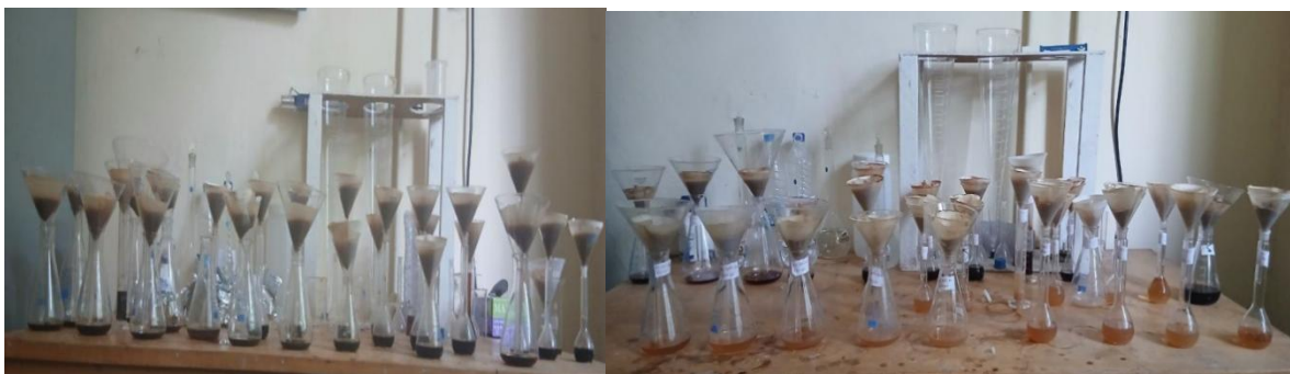
Figure 13: First stage hydrolysis sodium hydroxide followed by dilute acid hydrolysis filtration process.
