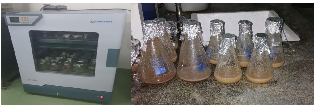
Figure 14: Second stage hydrolysis process using shaker incubator and SSF process Figure 15: Glucose content determination at 24h, 48h, and 72h
