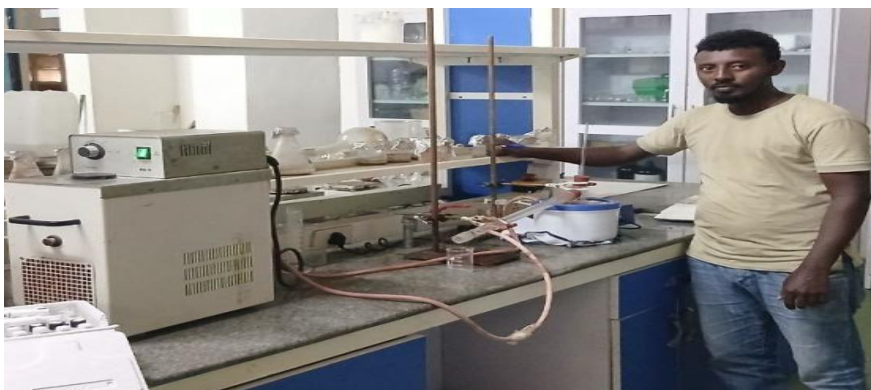
Figure 16: At distillation time to separate the fermented ethanol in to water at 78-80 0 c in analytical laboratory
