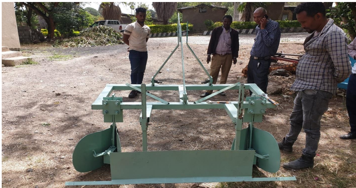
Figure 26. Rear view of the developed broad bed maker
