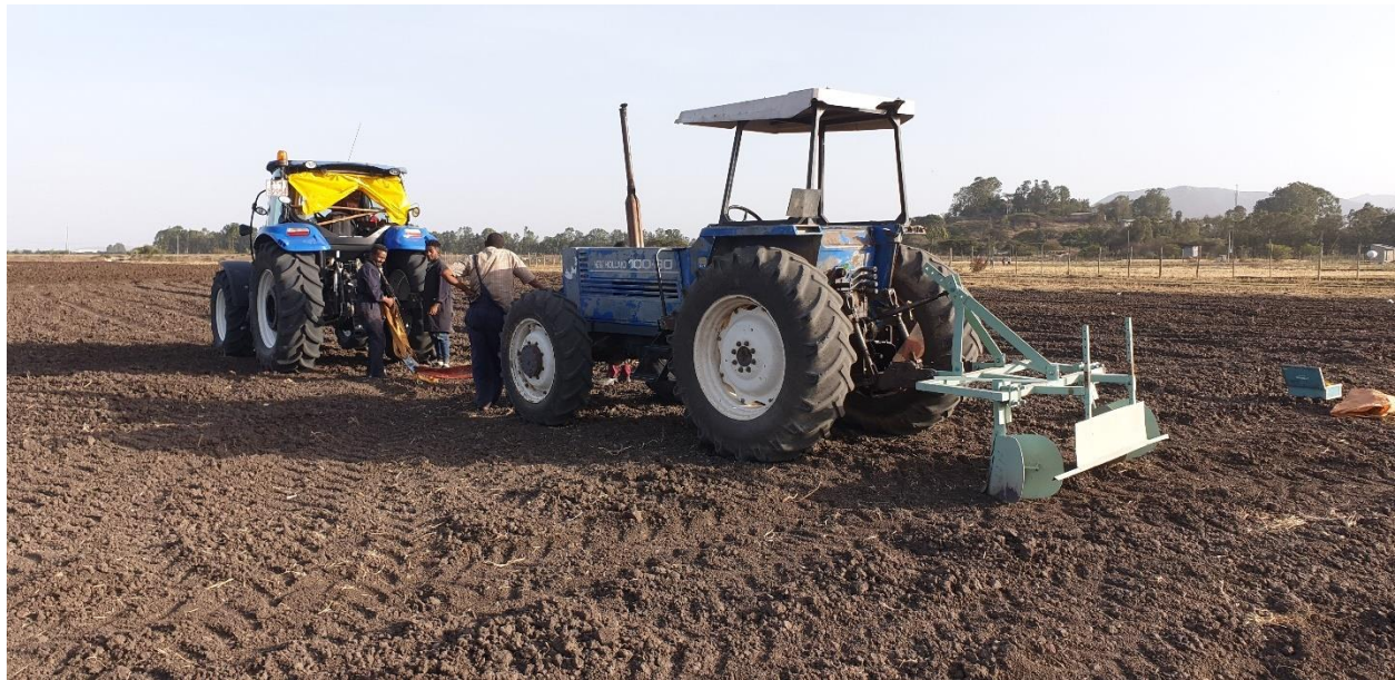
Figure 31. Measurement of the draft of broad-bed maker using dynamometer
