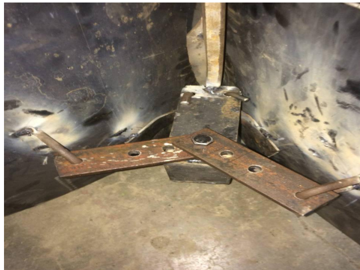
Figure 14. Size adjustment of the plough bottom
