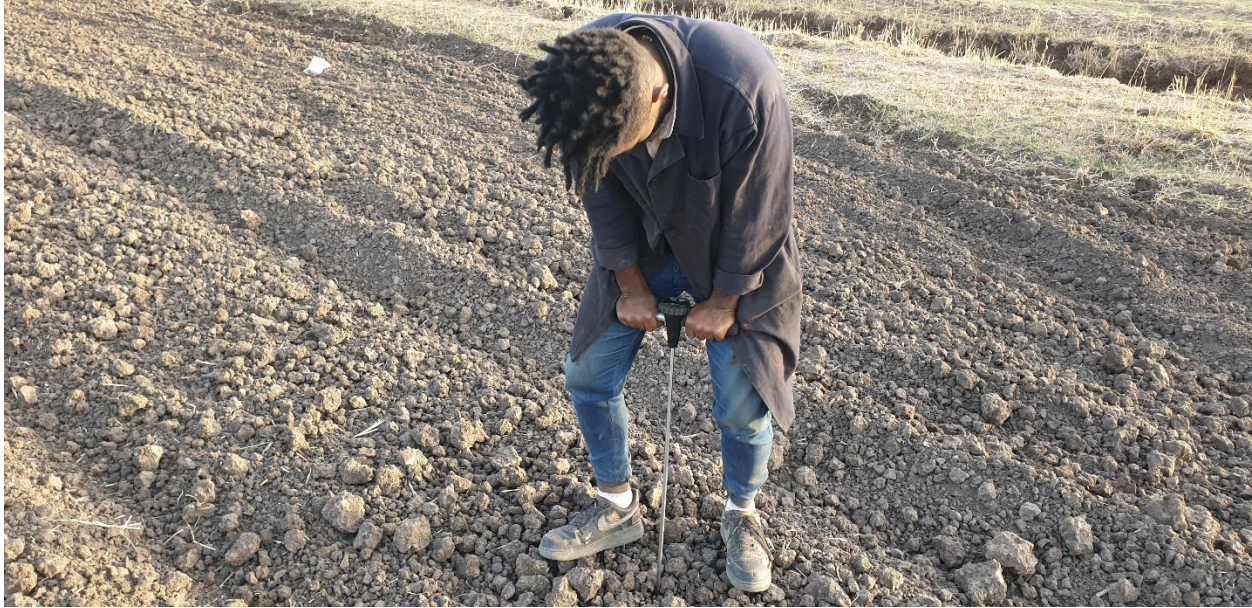
Figure 34. Soil penetration resistance test using cone penetrometer
