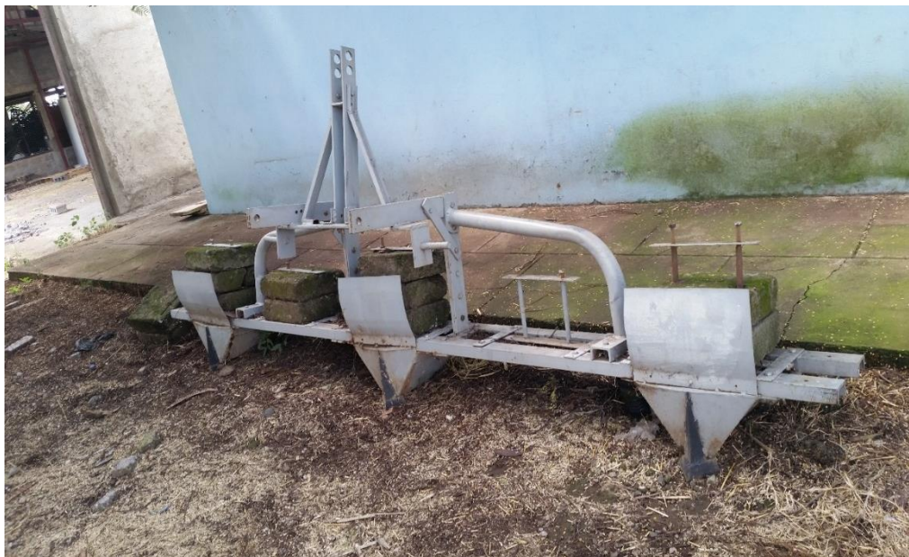
Figure 3. AIRIC made broad bed and furrow maker (Source: Photo taken by me MARC-AIRIC, Unpublished, 2013)
