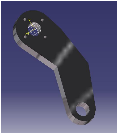
Figure 3. Catia drawing of brake actuator design with aluminum alloy material
