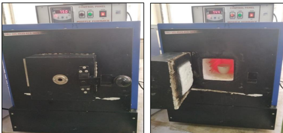
Figure 5.5: Adjusting muffle furnace and loading sample for TS of CC-BC450 Weigh the crucibles and add to each approximately 1 g, weighed to the nearest 0.1 mg, of the ground sample.
