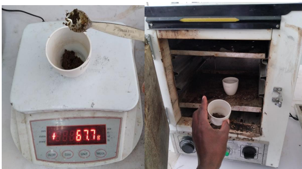
Figure 5.12: Weight and Loading of the crucible with the substrate for TS of CD
