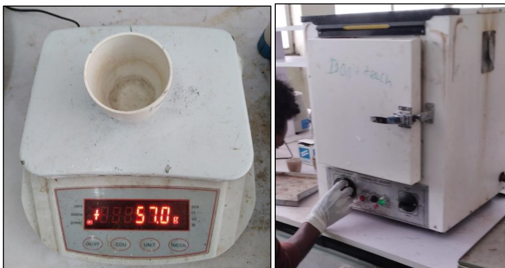
Figure 5.11: Weight of crucible after cleaning, heating, and adjusting oven for TS of CD 10g of freshly collected samples were weighed using an electrical balance (digital weight measuring device) and placed inside an electric hot air-oven maintained at 105°C using a crucible. The crucible was allowed to stay in the oven for 24 hours, then taken out, cooled to room temperature in a desiccator, and weighed.
