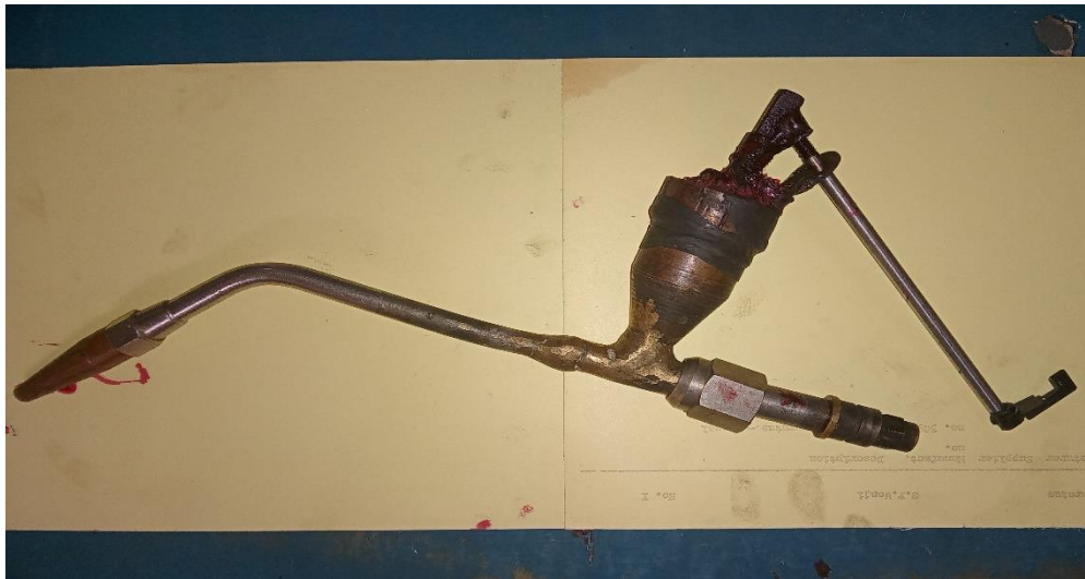
Figure 21 Modified oxy-acetylene cutting torch with powder supply and control valve
