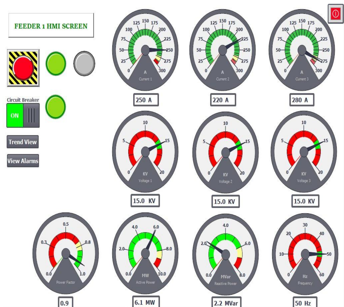
Figure 4. 12 HMI screen to monitor and control the real time substation status
