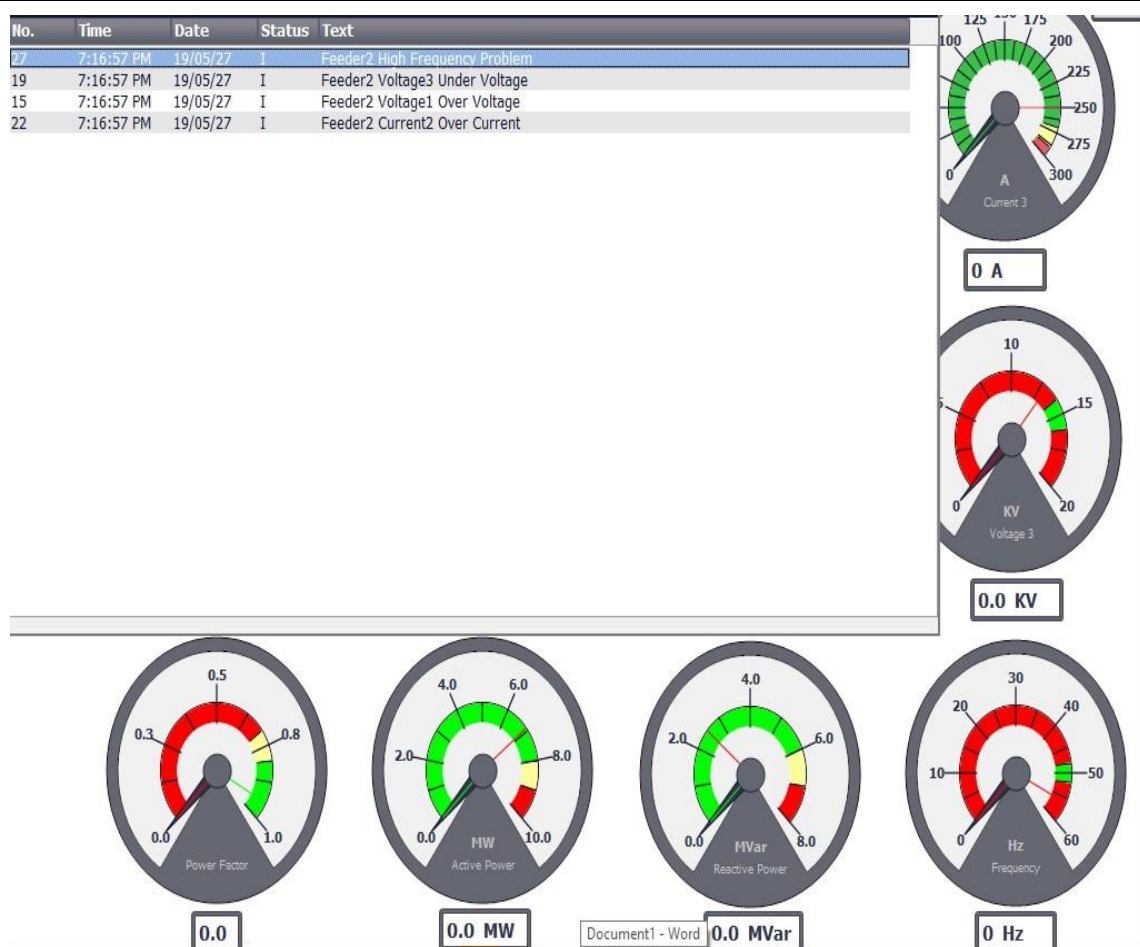
Figure 4. 29 Alarm text abnormal conditions
