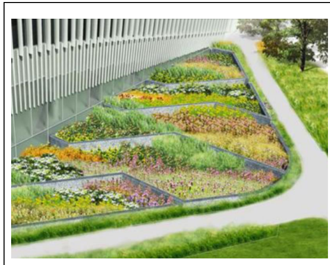
Figure 5.49: Visual reference of bio retention facility
