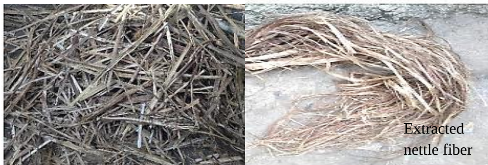
Figure 3. 3 Processing and collected nettle fiber product after processing
