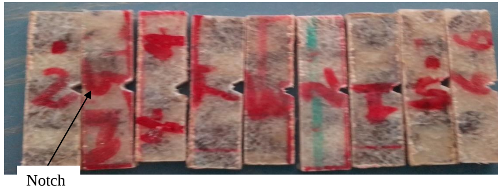
Figure 3. 22 Impact test specimen
