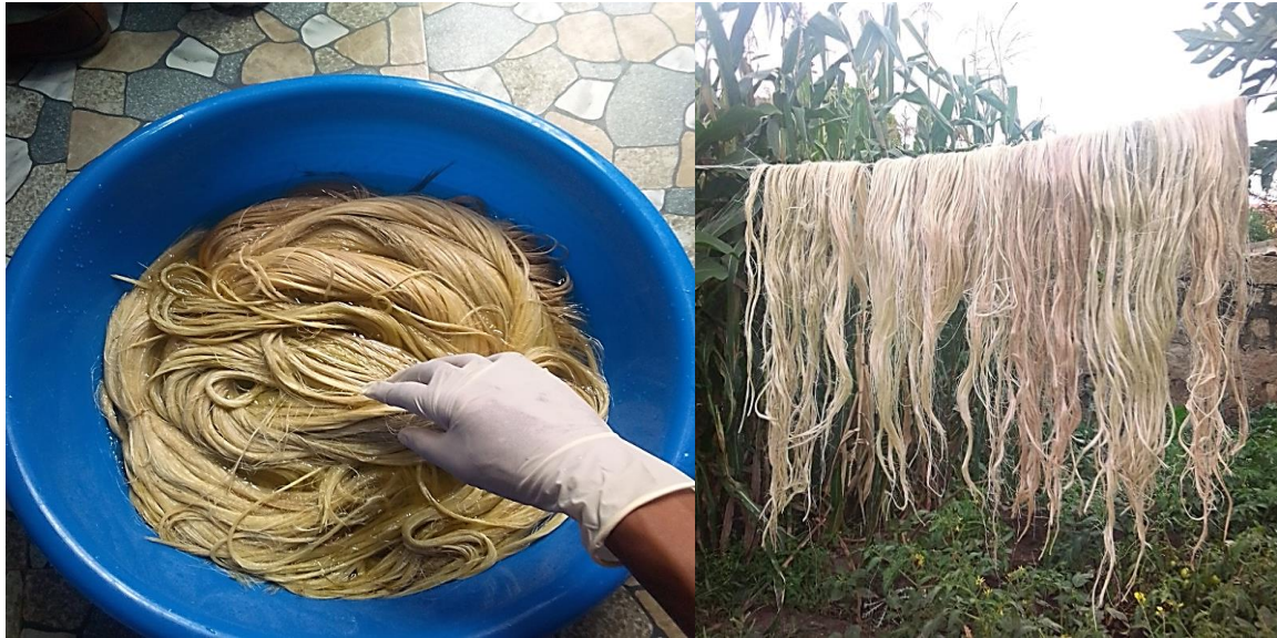
Figure 3. 9 Soaking sisal fiber in NaOH solution and drying in the sun
