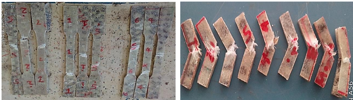
Figure 3.31: Specimen after tensile and impact test respectively
