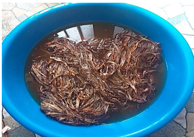
Figure 3. 4 Soaking nettle fiber into the water for further purifications
