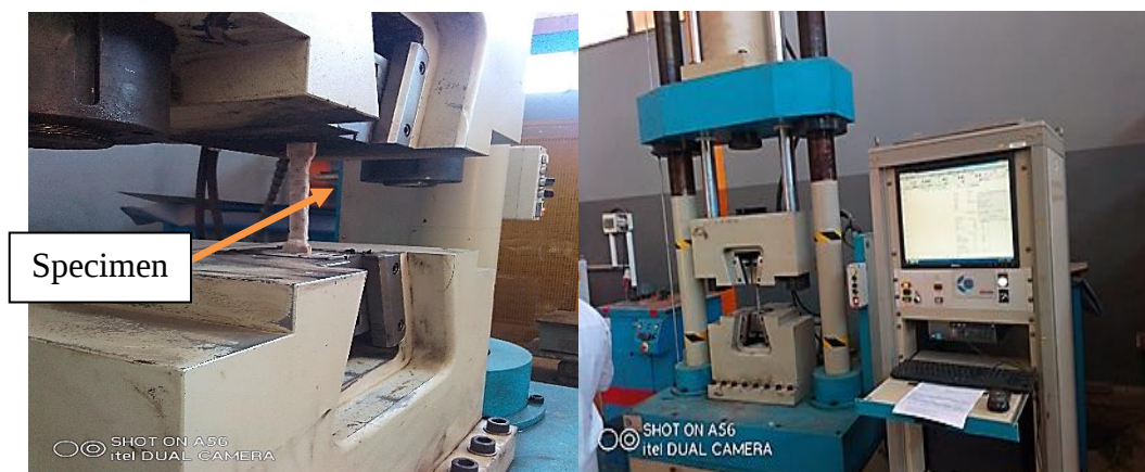
Figure 3. 20 UTM machine Sample loaded condition for tensile testing
