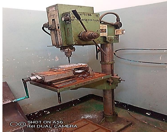
Figure 3. 29 Bench type drilling machine
