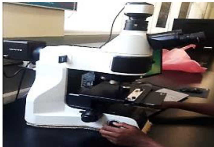
Figure 3. 25 Fixing of test condition for micro structure under optical microscope
