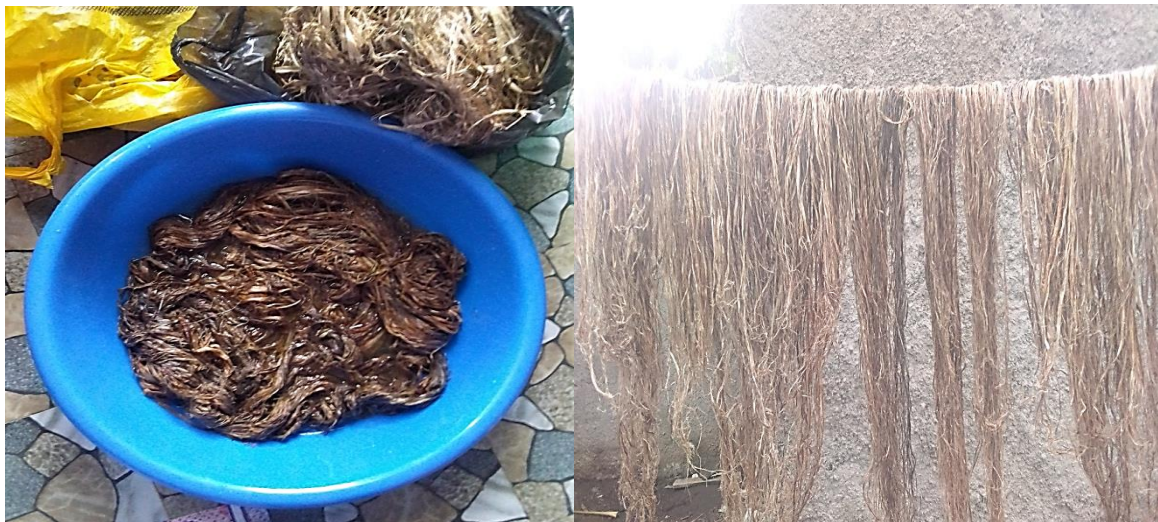
Figure 3. 8 Soaking nettle fiber in NaOH solution and drying it in the sun
