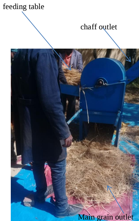
Figure 3.4.view of Melkassa made thresher (thresher I) illustrating main grain outlet, feeding table and chaff outlet.
