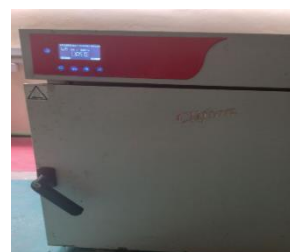
Dried in an oven at 105 °C for 24 hour
