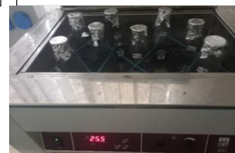
Shacked the flask at speed of 150 rpm at 25 °C for 24
