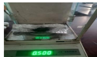
0.5g was measured and added to the solution
