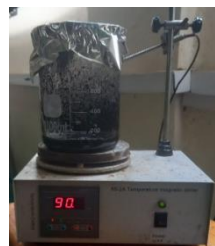
Stirred by magnetic stirrer for 2hr at 90 °C
