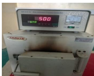
Calcination (Muffle furnace) at (300- 700 °C)
