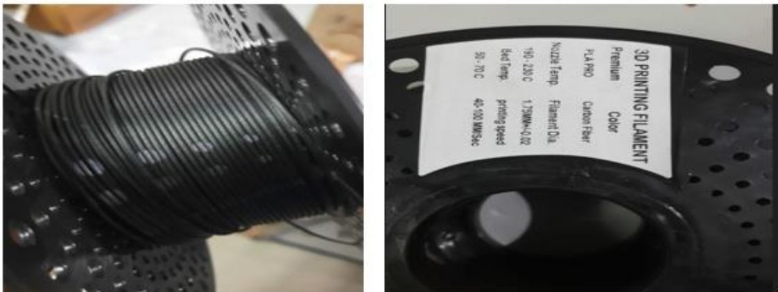
Figure 3-2: Carbon fiber reinforced polyamide 6 filament
