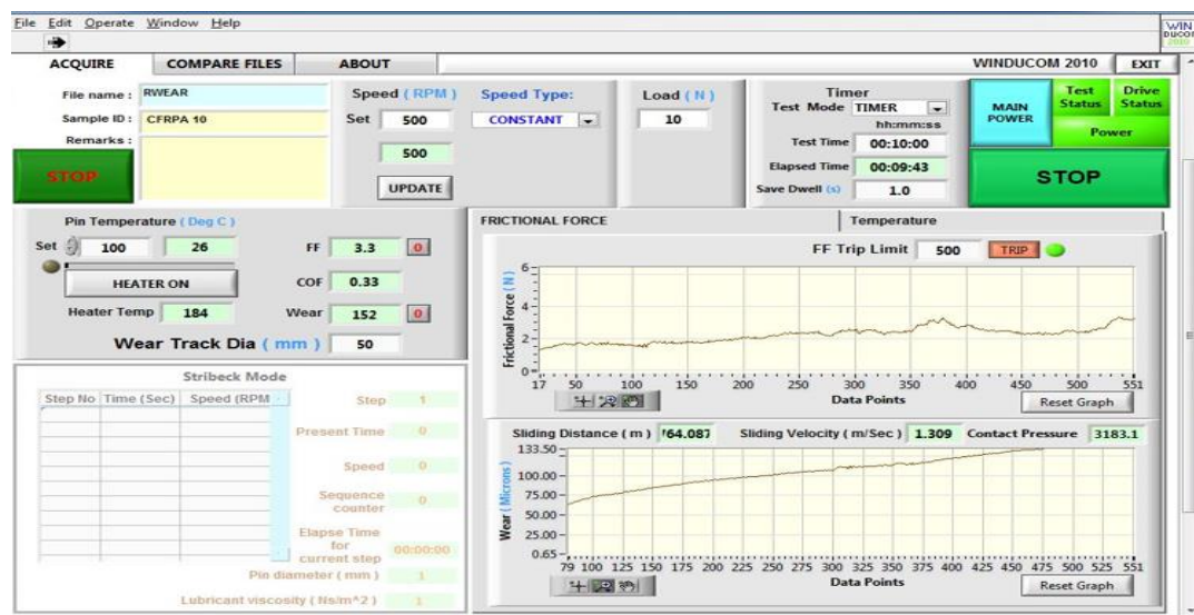
Figure A-2: Graph of the wear test setup
