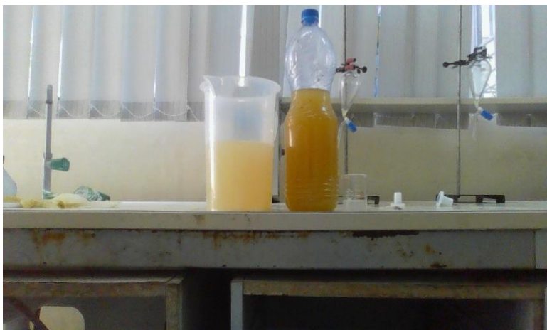
Figure 4.6: Biodiesel product after washing and drying
