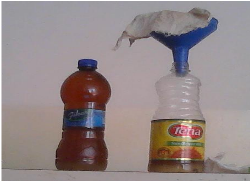
Figure 3.2: Filtering of waste cooking oil to removes slag and impurities
