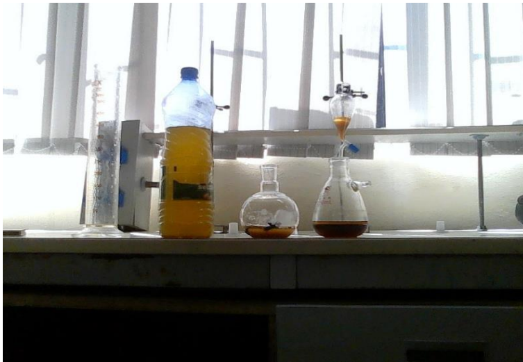
Figure 4.5: Biodiesel product before washing and drying
