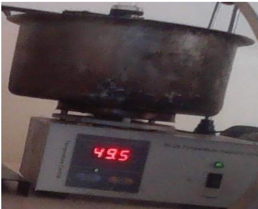
Figure 3.3: Heating of the waste oil to avoid moisture
