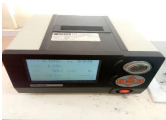
Figure 4.12: Flue gas analyzer
