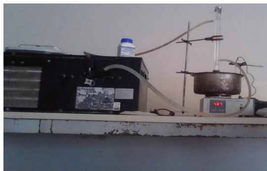
Figure 4.1: Reactor setup with chiller used for the transesterification of waste oil
