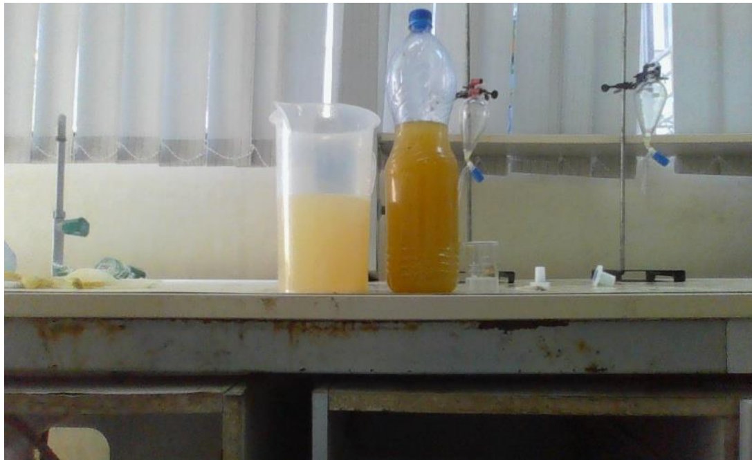
Figure 3.4: Amber-yellow biodiesel after washing
