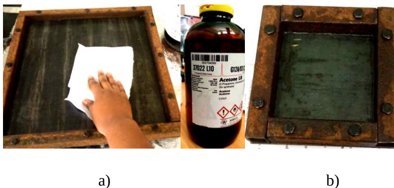
Figure 3. 4 Preparation of mold a) Cleaning mold 2 (larger mold 300x300x30mm) with laboratory grade acetone, b) Petroleum jelly applied on mold 1 (Smaller mold 100x100x30mm).
