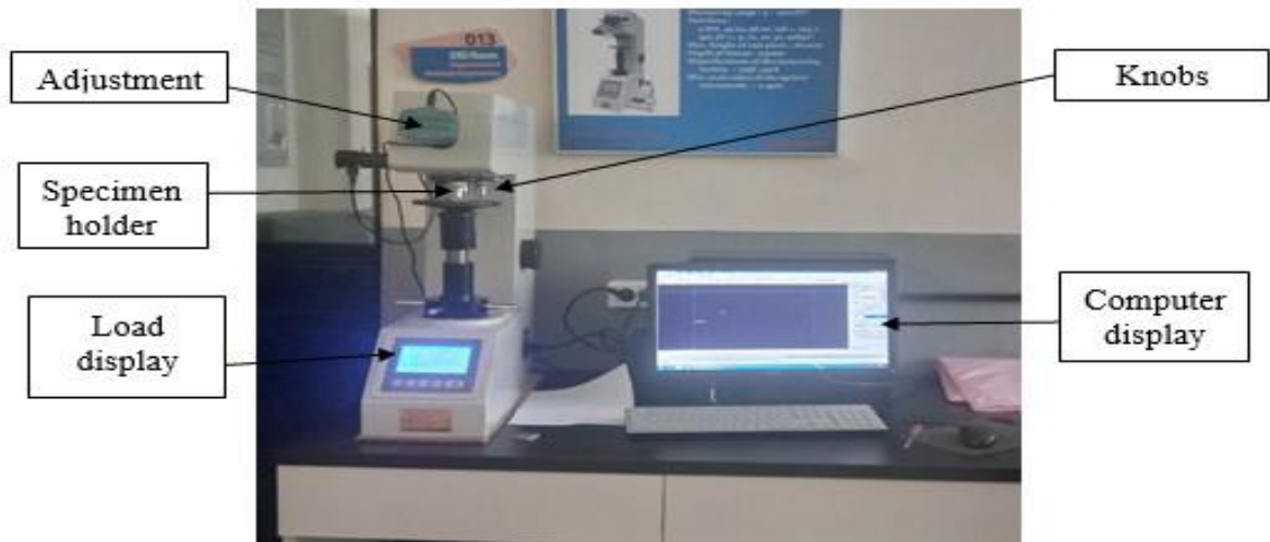
Figure 3. 15 Hardness test setup
