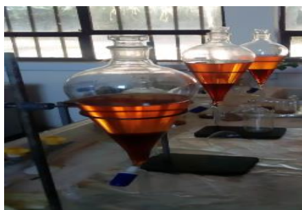
Figure 3.7: Separation of biodiesel and glycerol
