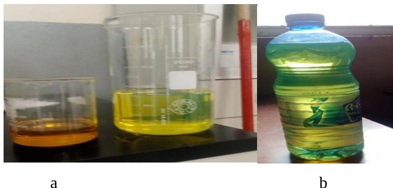
Figure 3.12 (a) Measured diesel and biodiesel and (b) Diesel-biodiesel blend
