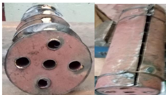
Frontal views of heat exchanger
