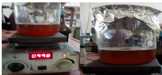
Figure 3.6: Heating the mixtures of KOH and methanol with oil
