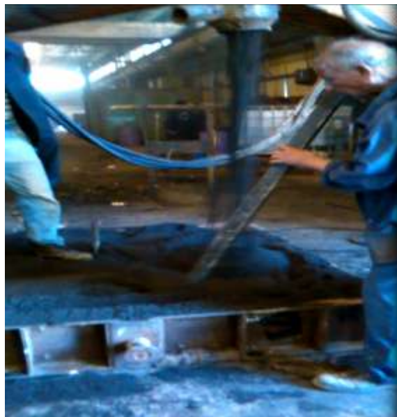
Figure-6.5 Ramming practice in the foundry
