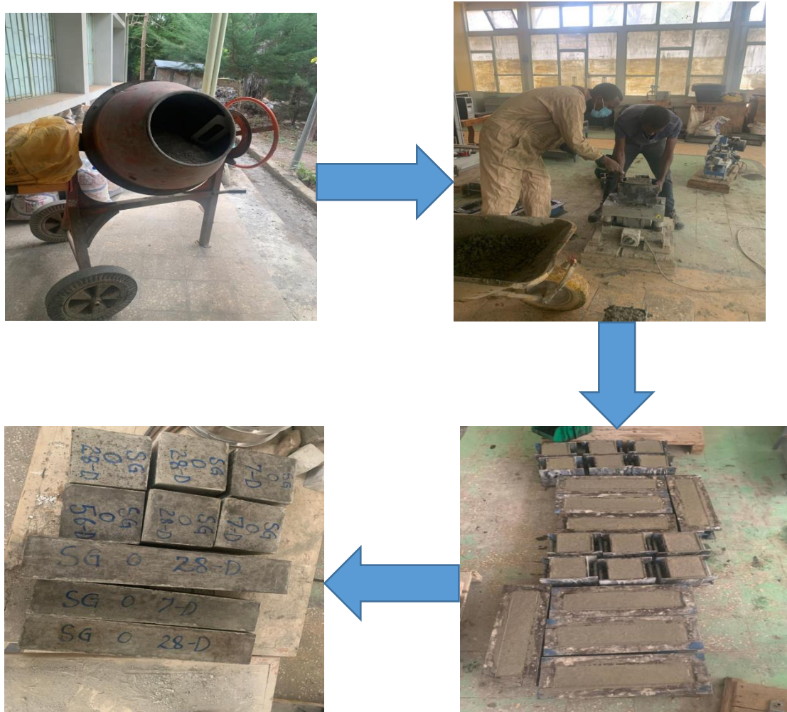
FIGURE 3. 4 Concrete Mixing and Specimen Preparation
