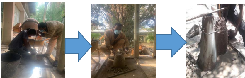
FIGURE 3. 5: Process of measuring a slump value from Slump Test
