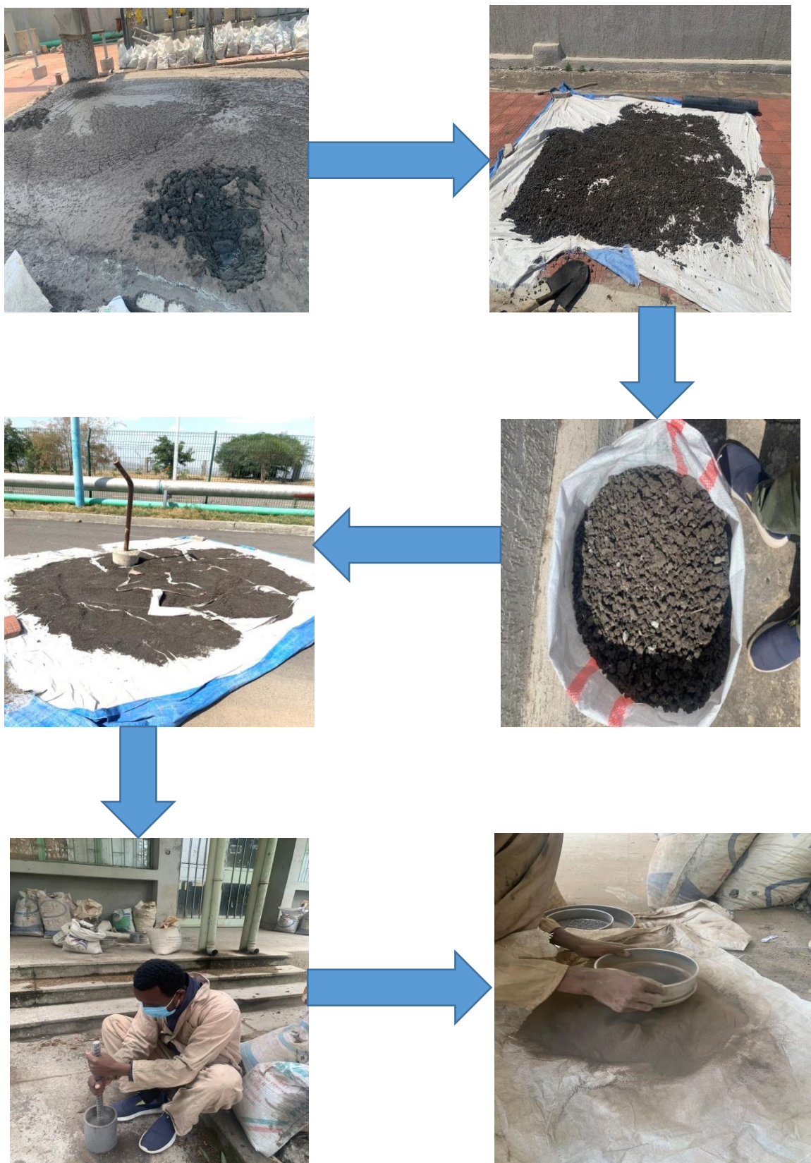
FIGURE 3. 3 Collection and Preparation of Dried Sludge powder
