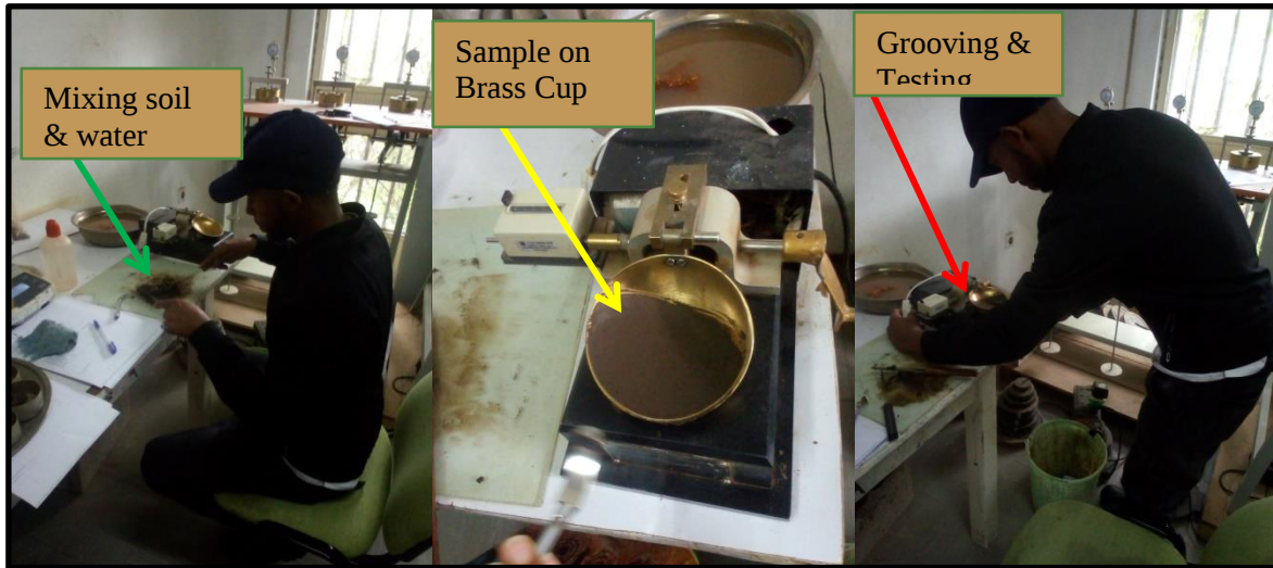
Figure 13 Liquid limit test using digital casagrande apparatus.
