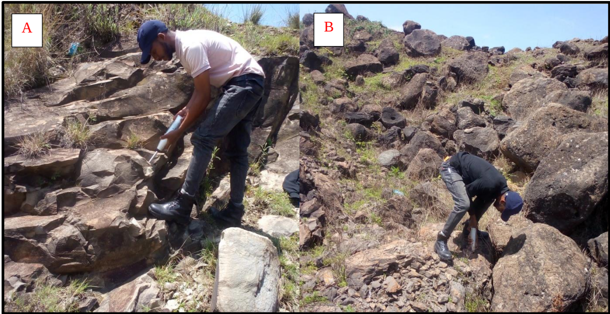
Figure 11 Insitu strength measurement using schmidit hammer on ignimbrite rock (A) and on fractured basalt rocks (B).
