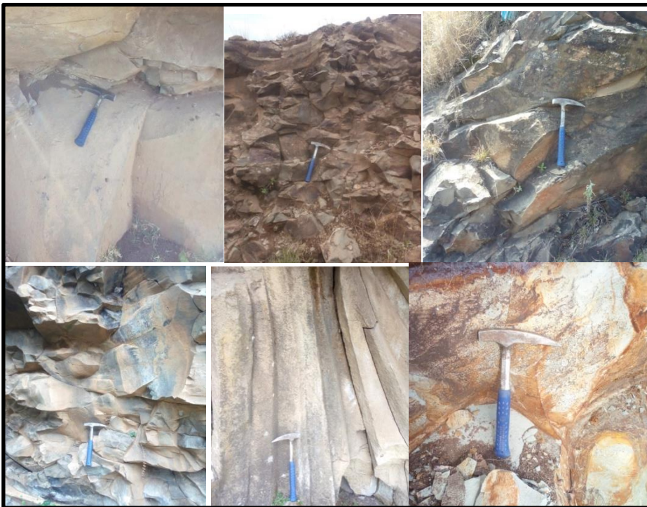
Figure 18 Ignimbrite rock with different fracture and weathering rate.
