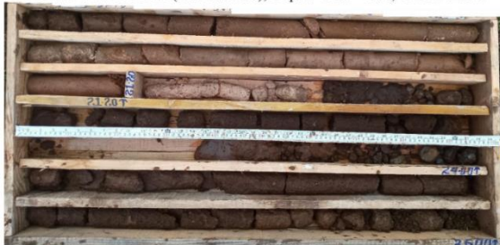
Proj :- Ashebaka D. & I. Project BH.ID :- ASHBH-03 (R. Abutment), Depth:- 19.0 - 26.0, Box # 4 of 7
