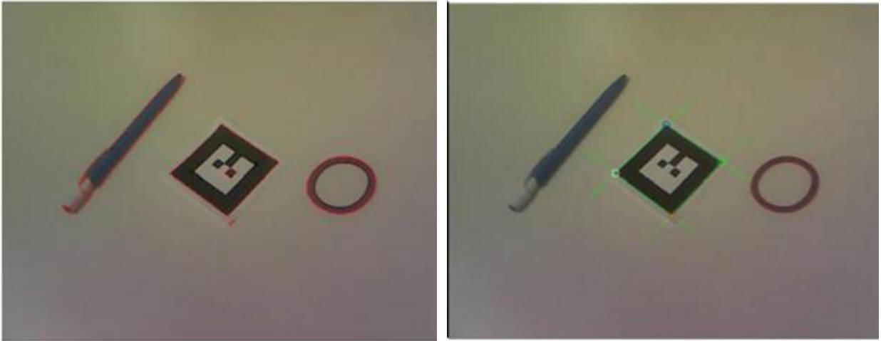
Figure 2.2. Marker Detection using the CV algorithm (Siltanen, 2012)
