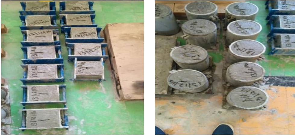
Figure 4: Casting of cube and cylindrical specimens
