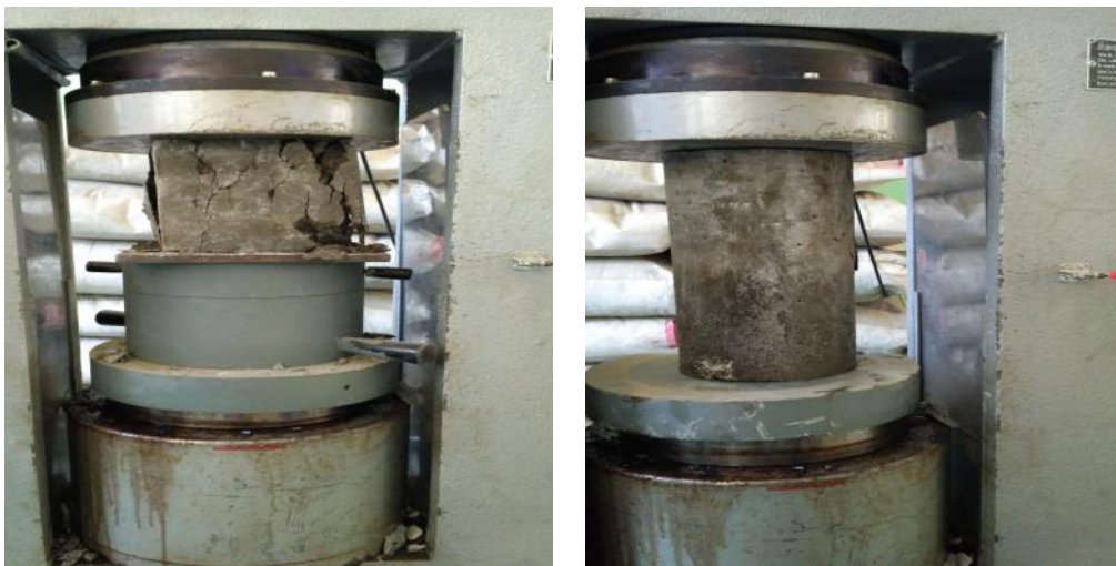
Figure 7: Set up for compressive strength for cube and cylinders.
