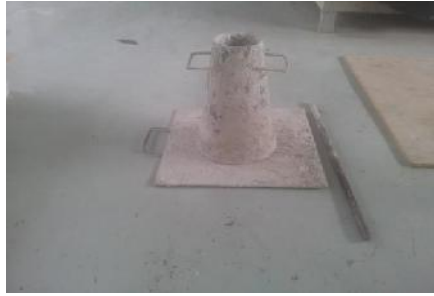
Figure 6: Slump cone test apparatus
