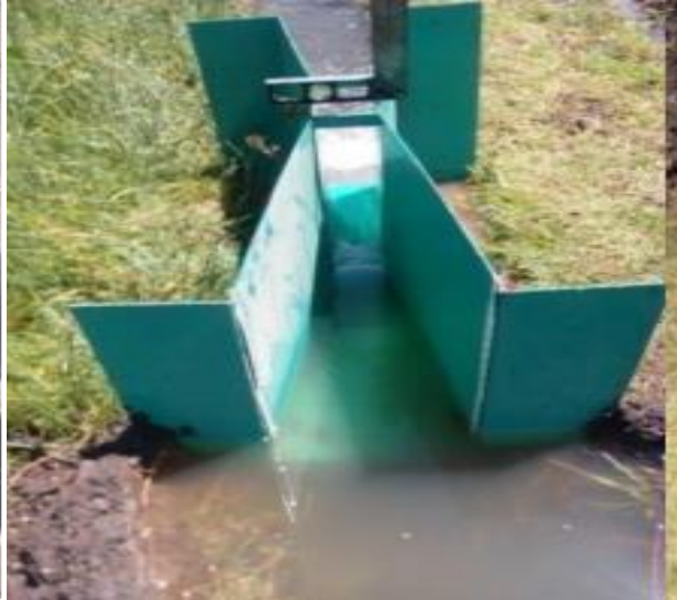
partial flume inlet
