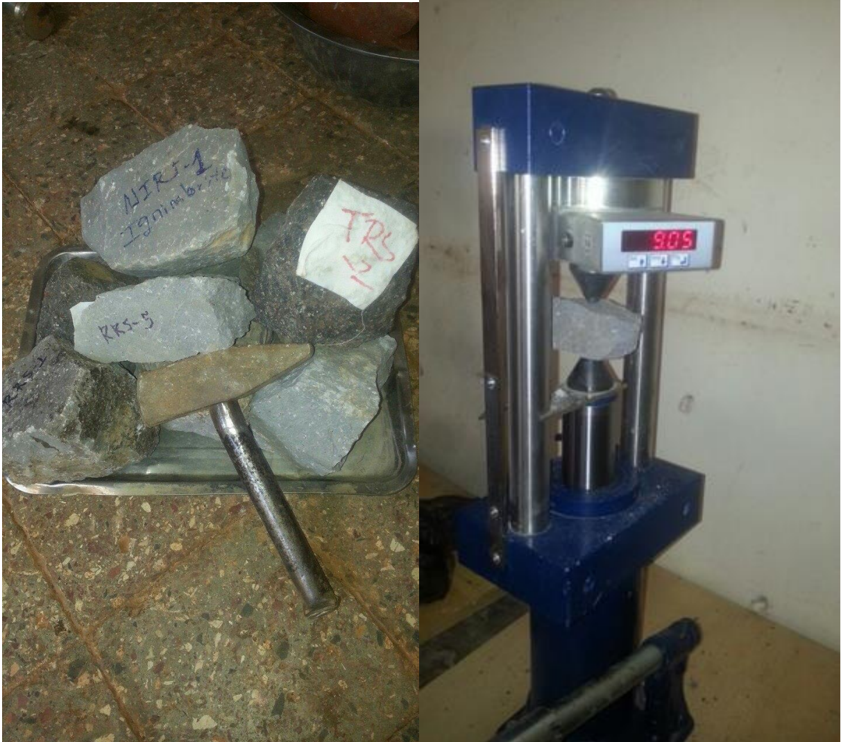
Figure 3.3: Irregular sample taken from critical slope section of quarry and point load test.
