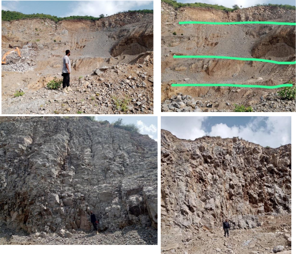
Figure 3.1: Structural and non-structural slope section of quarry site that have highly jointed and create steep cut slope due to quarrying operation.
