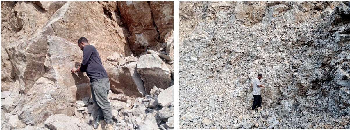
Figure 3.2: In-situ strength test using Schmidt hammer at different critical slope section of quarry
