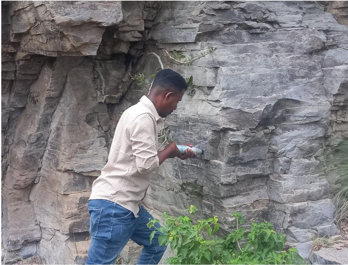
Figure 3. 2 In-situ strength test of rock determination of rebound values.
