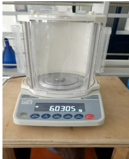
Figure 3.2 Weight in air of a compacted chip of aspect ratio 25.4/7
