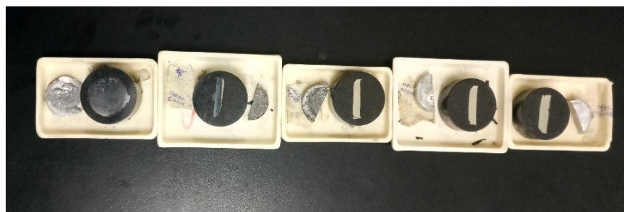
Figure 3. 8 Prepared samples passing mounting, grinding, polishing and re-polishing steps.
