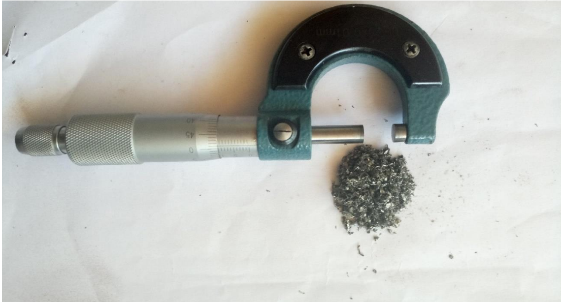
Figure 3.1 Chips prepared for friction stir consolidation process
