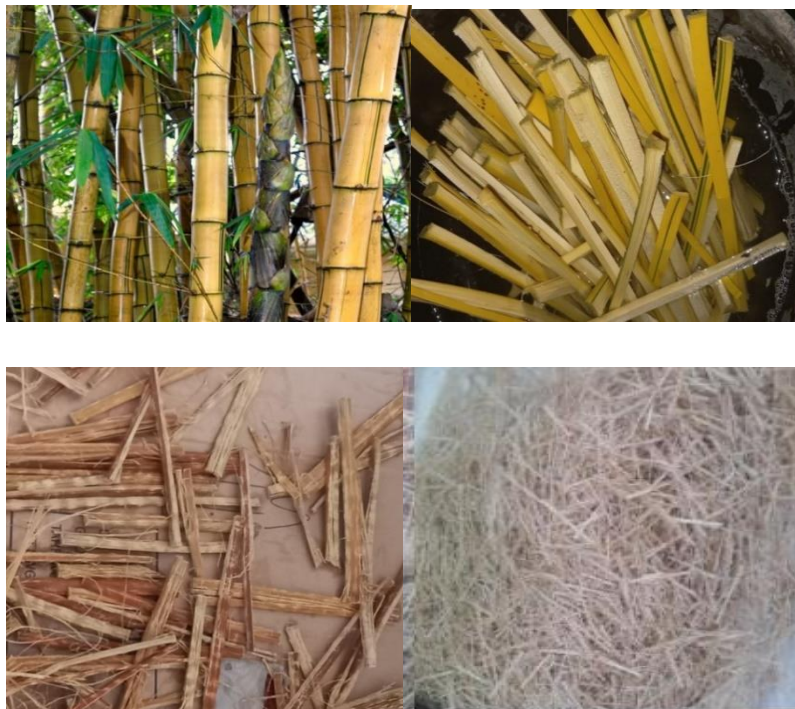
Figure 3.5: Extraction process of Bamboo Fibers
