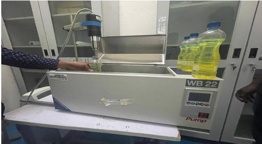
Figure 3. 11. Made dissolve with fuel and Iron (III) oxide ( \text{Fe}_2\text{O}_3 ) nanoparticle
