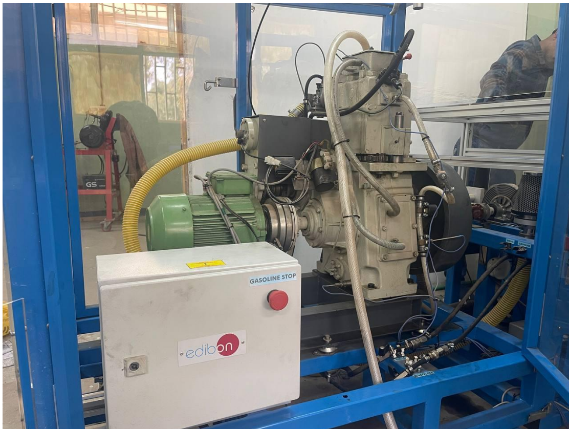
Figure 3. 2. Photographic view of TM 12-01 engine experimental setup
